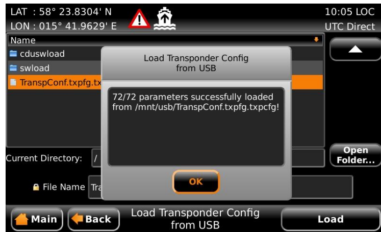
Figure 46 – Transponder Config successfully loaded.
