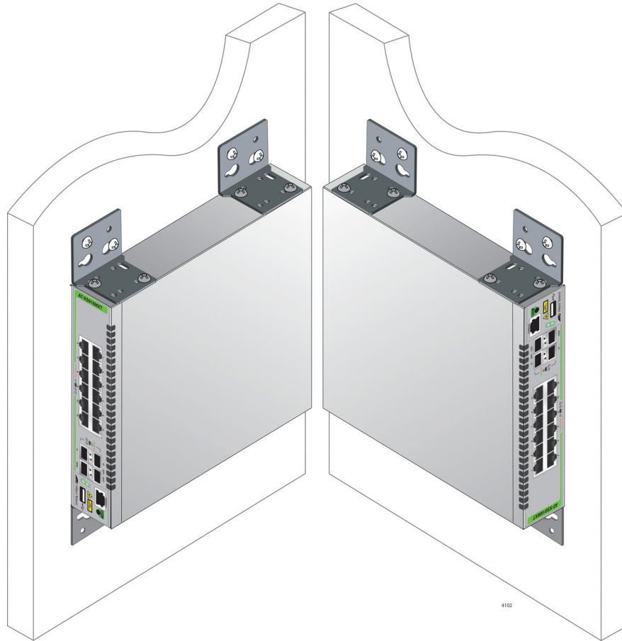
Figure 16. Positions of the XS916MX Series Switch on a Wall
