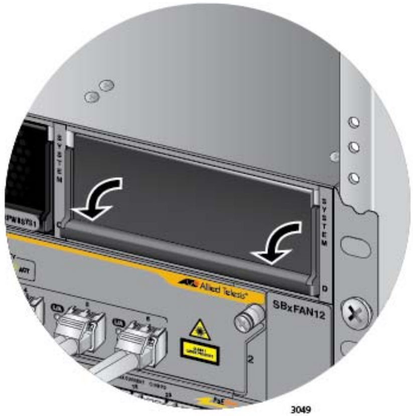
Figure 148. Lowering the Locking Handle on the Power Supply Slot Cover
