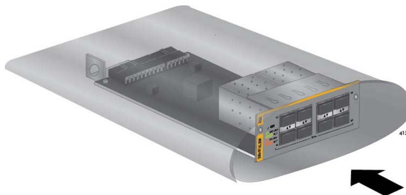
Figure 164. Storing the Expansion Module in an Anti-static Bag
