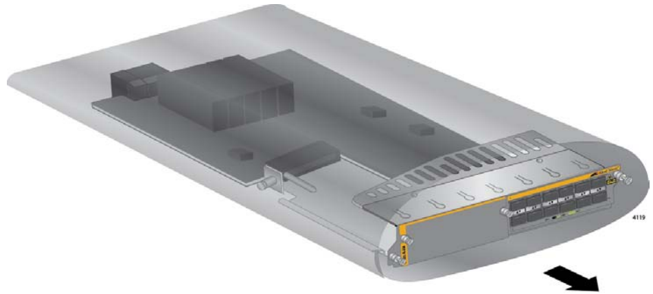
Figure 72. Removing the AT-SBx81XLEM Line Card from the Anti-static Bag
