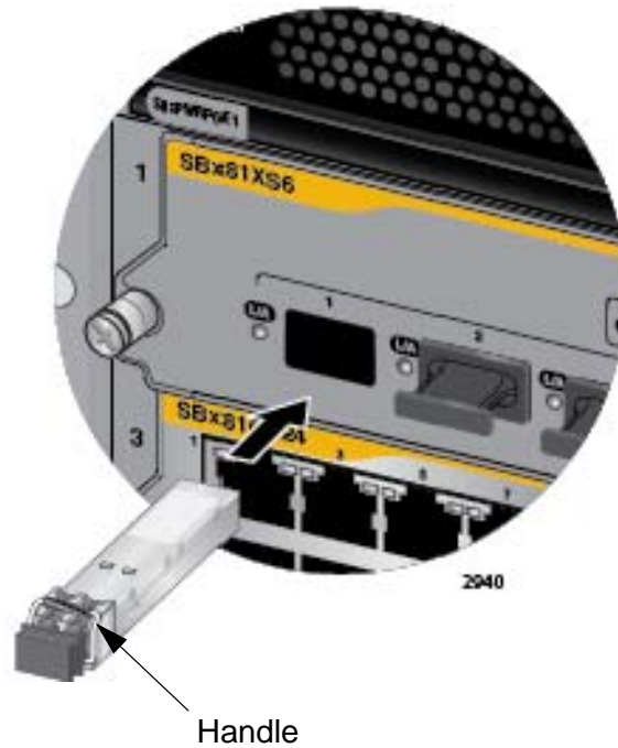
Figure 95. Installing an SFP+ Transceiver in the AT-SBx81XS6 Line Card
