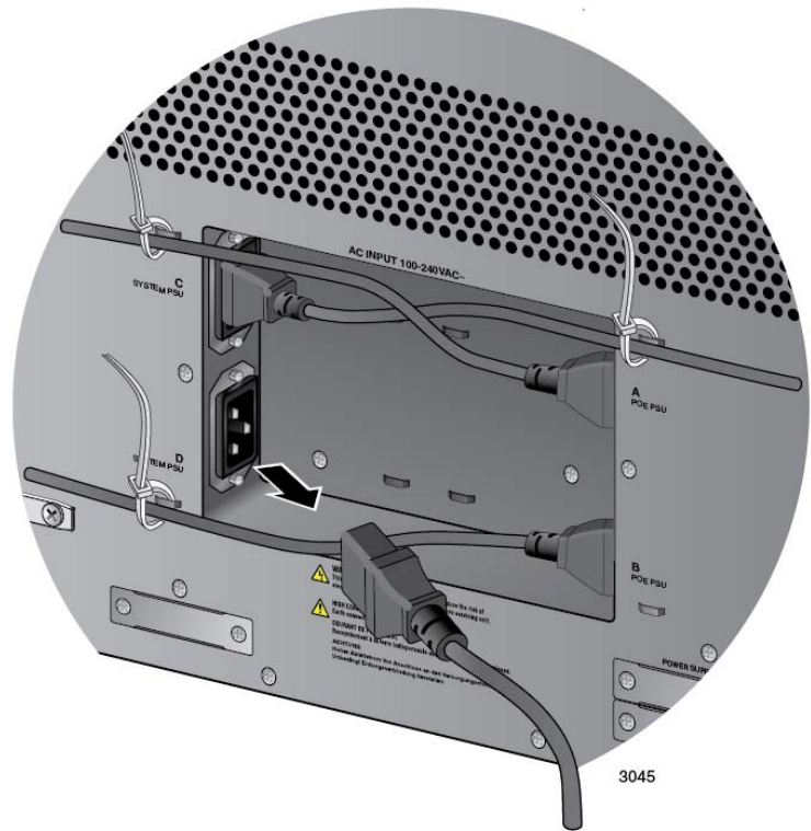
Figure 144. Disconnecting the AC Power Cord from the AC Socket on the Back Panel
