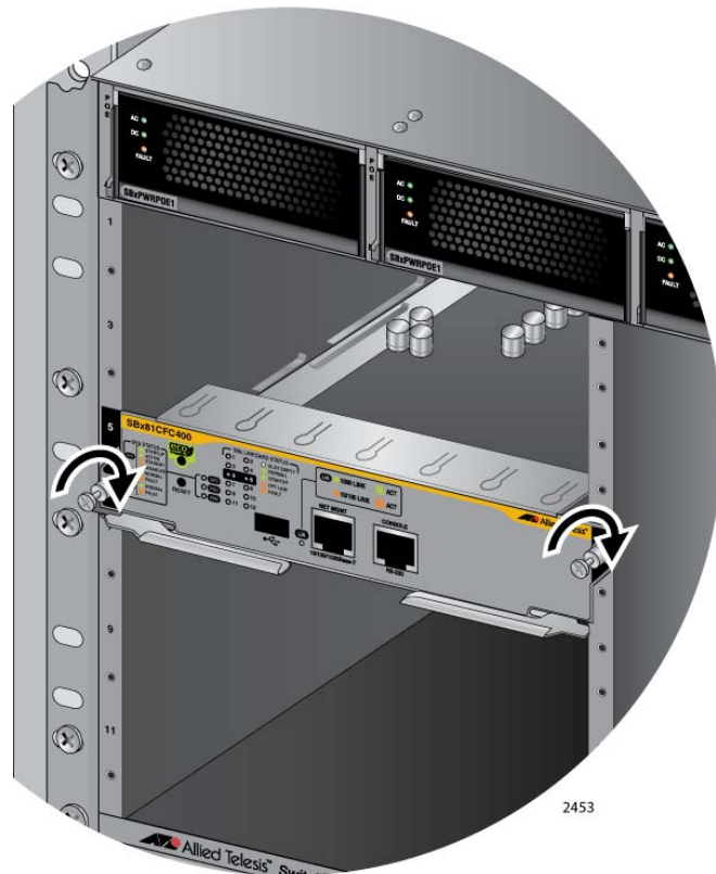
Figure 71. Tightening the Thumb Screws on the AT-SBx81CF400 Card
