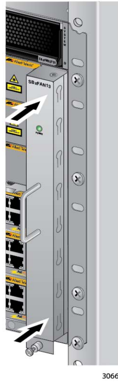
Figure 173. Securing the AT-SBxFAN12 Fan Module on the Backplane Connector
