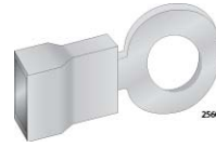
Figure 111. Grounding Wire Terminal
