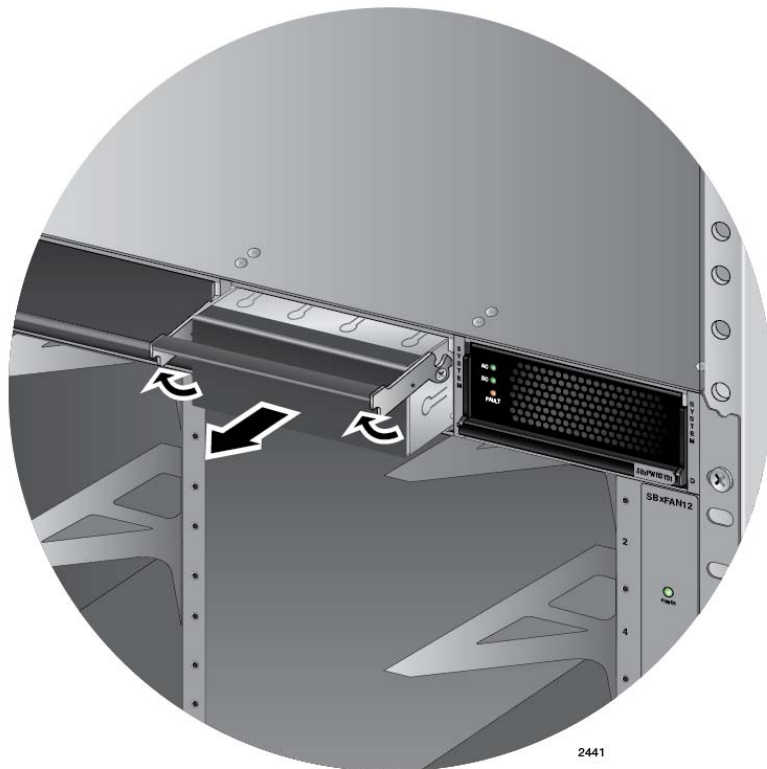
Figure 46. Removing the Blank Slot Cover from Power Supply Slot C
