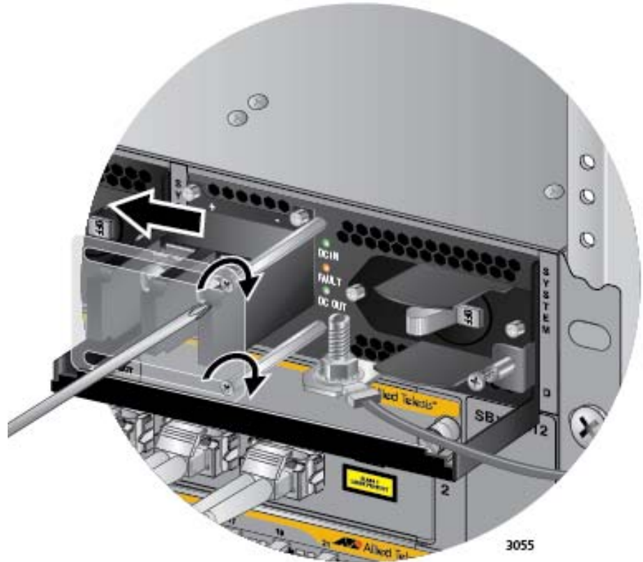
Figure 154. Closing the Plastic Cover
