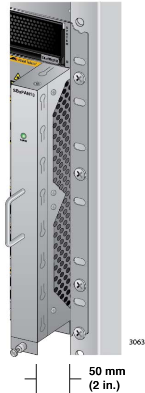
Figure 170. Withdrawing the AT-SBxFAN12 Fan Module 51 mm (2 In.) from the Chassis
