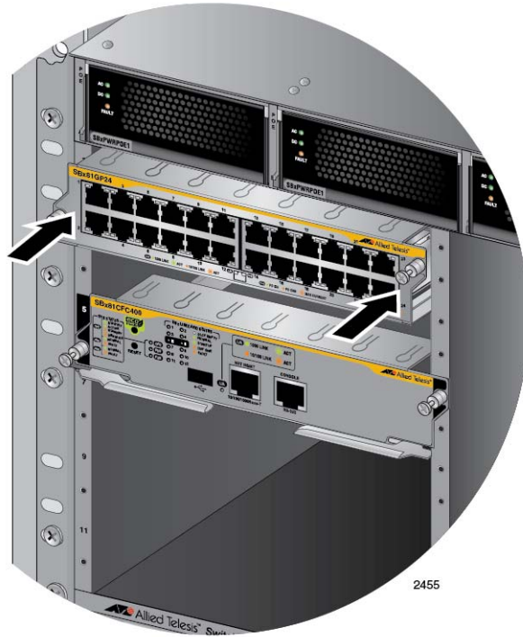
Figure 87. Seating an Ethernet Line Card on the Backplane Connector
