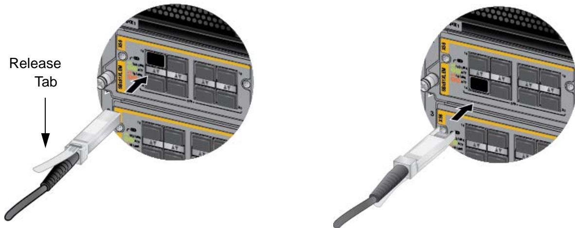
Figure 101. Installing the AT-SP10TW Cable in the AT-SBx81XLEM/XS8 Expansion Module
