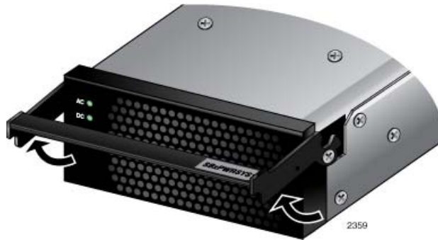
Figure 48. Unlocking the Handle on the Power Supply
