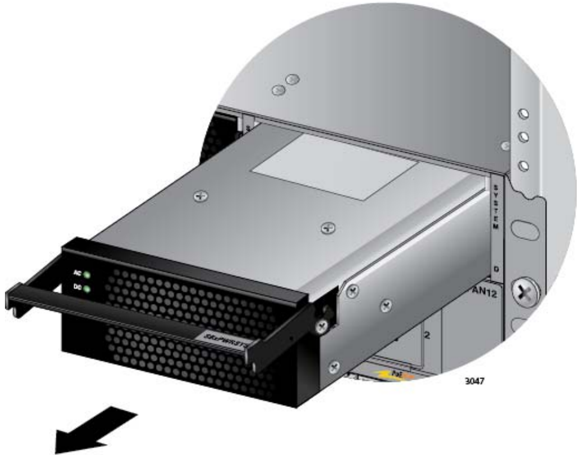
Figure 146. Removing the Power Supply from the Chassis
