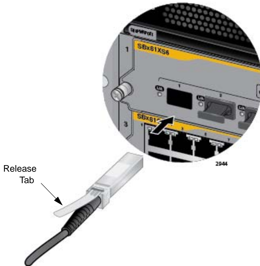
Figure 100. Installing the AT-SP10TW Cable in the AT-SBx81XS6 Line Card
