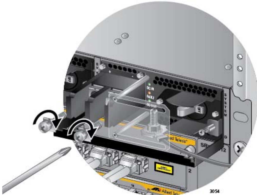
Figure 153. Reinstalling the Screws on the Positive and Negative Terminals
