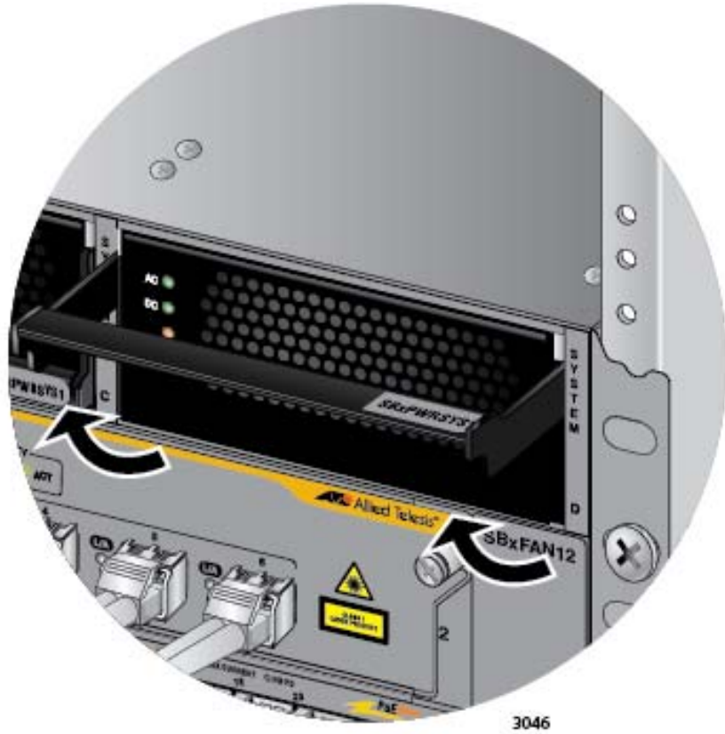
Figure 145. Lifting the Locking Handle on the Power Supply
