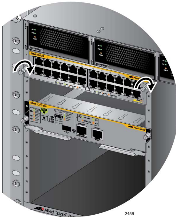
Figure 88. Tightening the Thumb Screws on an Ethernet Line Card
