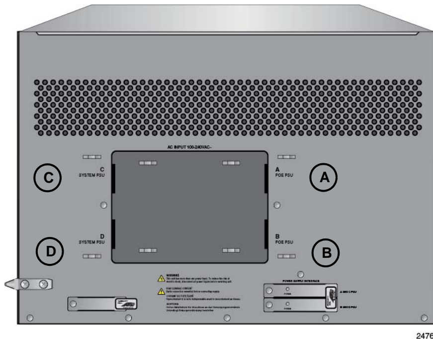
Figure 104. AC Sockets on the Rear Panel of the AT-SBx8112 Chassis
