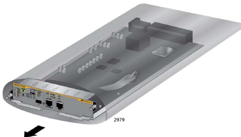
Figure 60. Removing the AT-SBx81CF400 Controller Fabric Card from the Anti-static Bag
