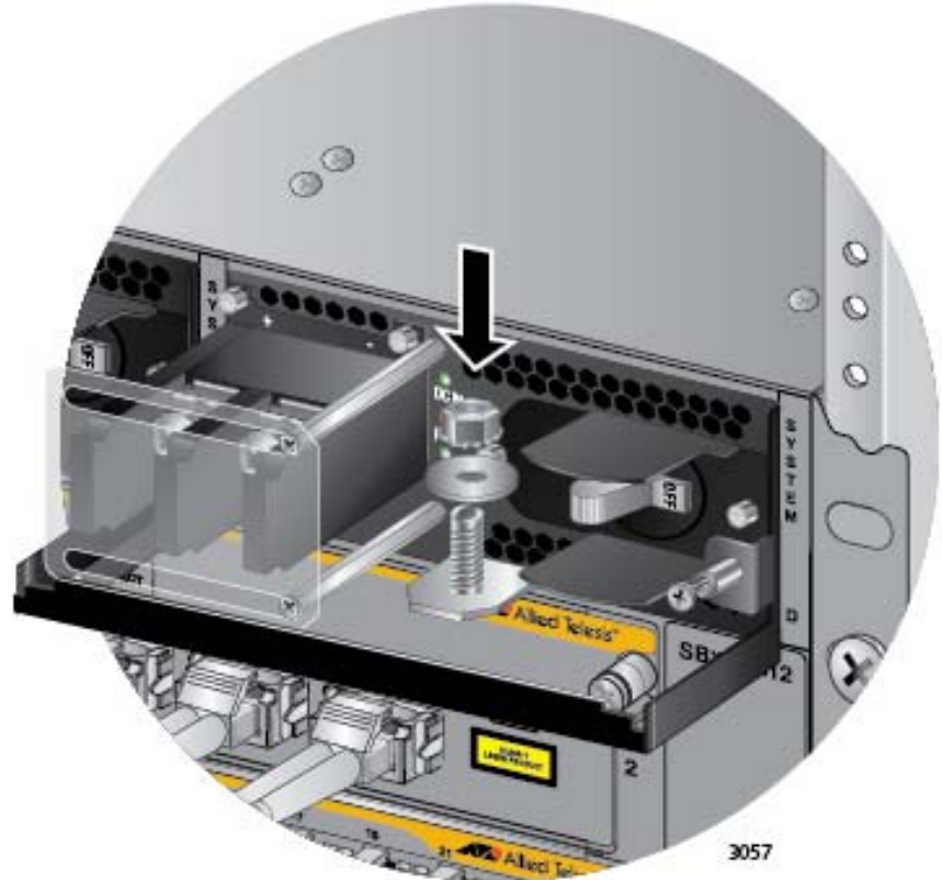
Figure 141. Reinstalling the Nut and Washer on the Grounding Post
