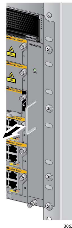
Figure 146. Loosening the AT-SBxFAN12 Fan Module from the Backplane Connector
