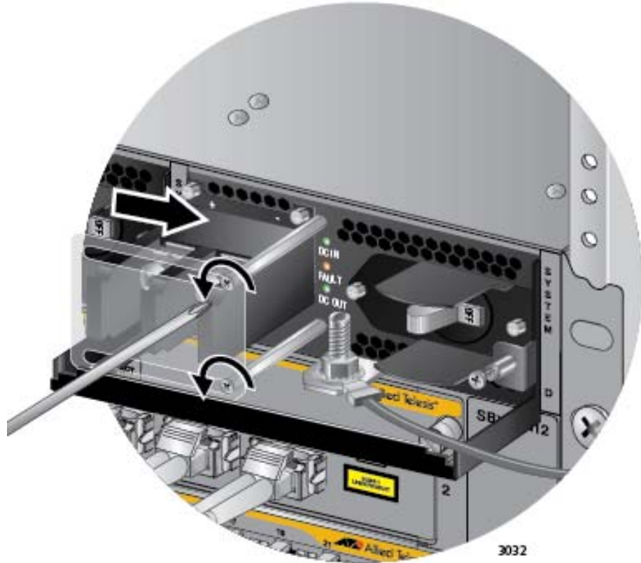
Figure 108. Opening the Plastic Cover
