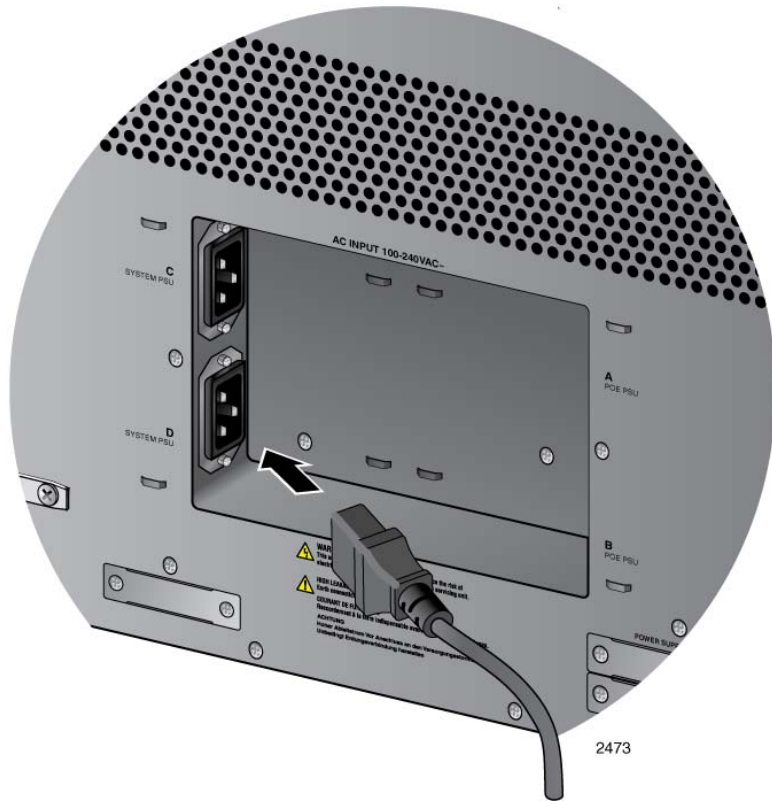
Figure 90. Connecting the AC Power Cord for the AT-SBxPWRSYS1 or AT-SBxPWRSYS2 AC System Power Supply
