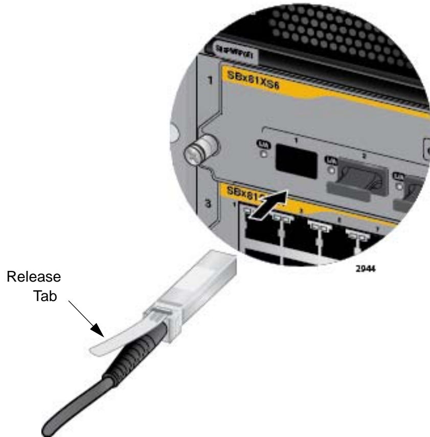
Figure 88. Installing the AT-SP10TW Cable in the AT-SBx81XS6 Line Card
