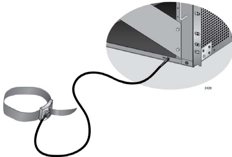
Figure 38. ESD Socket and Wrist Strap
