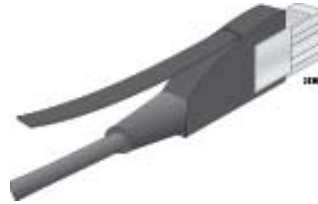
Figure 73. RJ Point 5 Cable Connector for AT-SBx81GT40 Line Card
