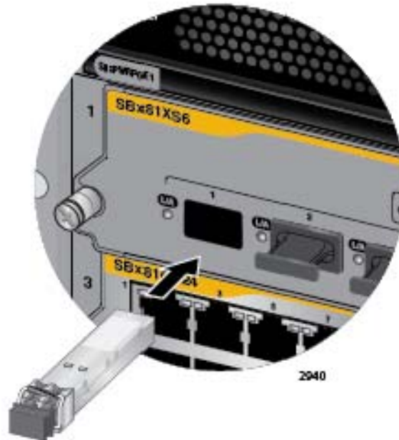
Figure 83. Installing an SFP+ Transceiver in the AT-SBx81XS6 Line Card
