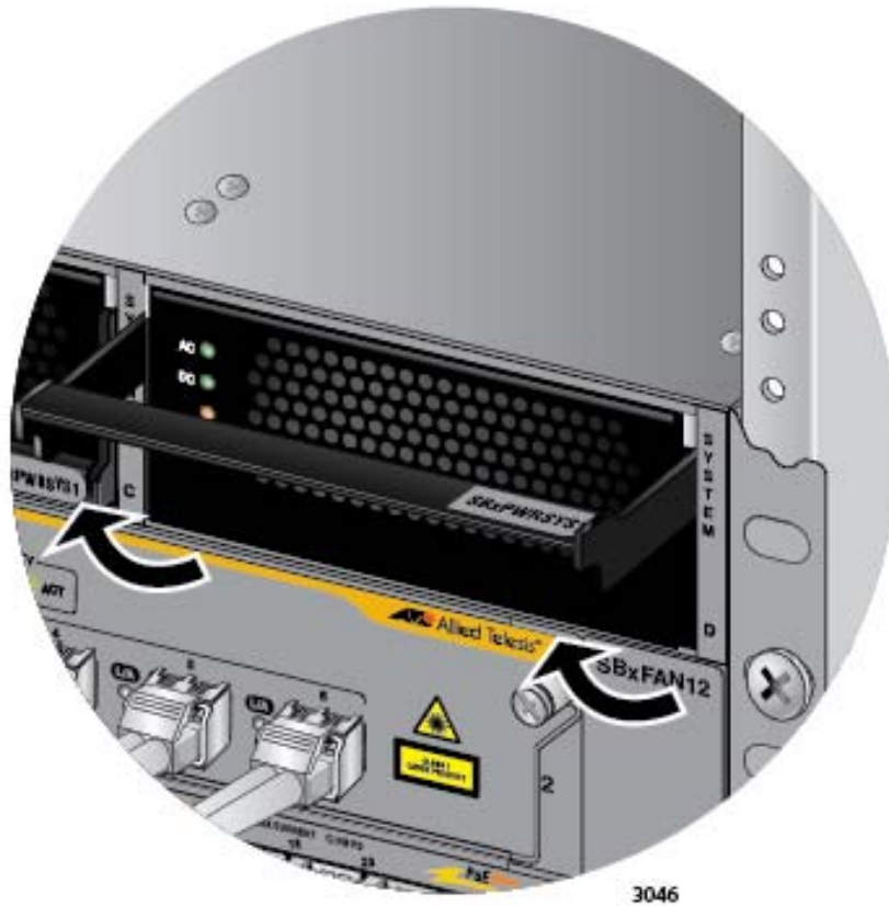
Figure 130. Lifting the Locking Handle on the Power Supply
