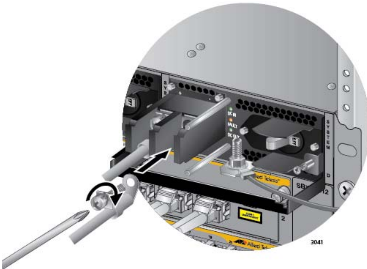
Figure 119. Connecting the Negative (-) Power Wire with a Right Angle Terminal
