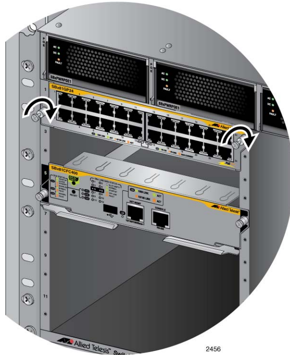
Figure 70. Tightening the Thumb Screws on an Ethernet Line Card
