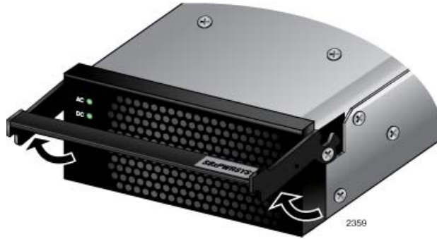
Figure 42. Unlocking the Handle on the Power Supply
