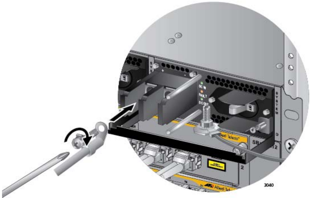
Figure 118. Connecting the Positive (+) Power Wire with a Right Angle Terminal
