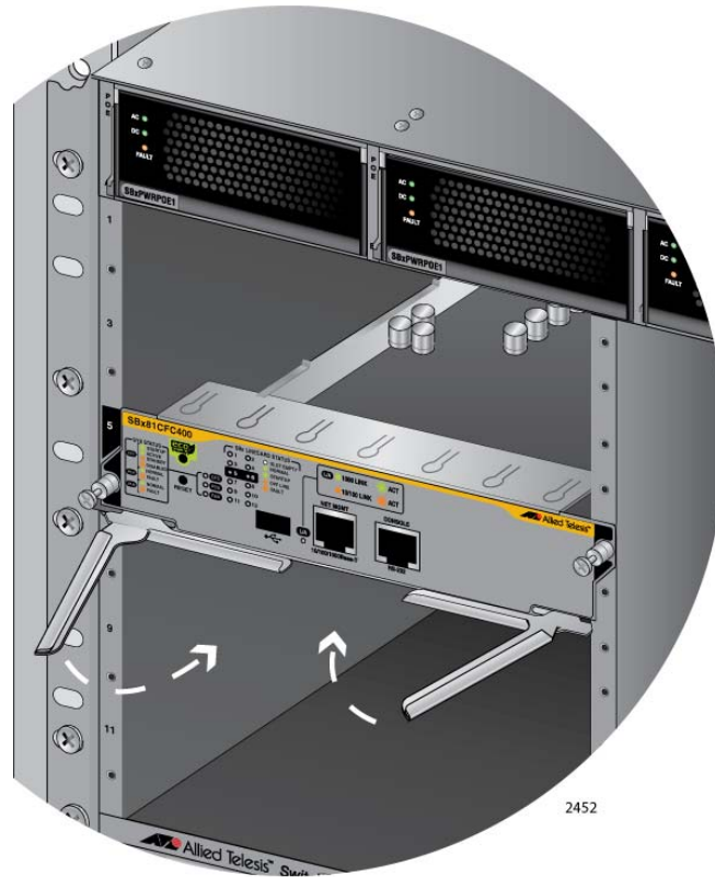
Figure 64. Closing the Locking Levers on the AT-SBx81CF400 Controller Fabric Card
