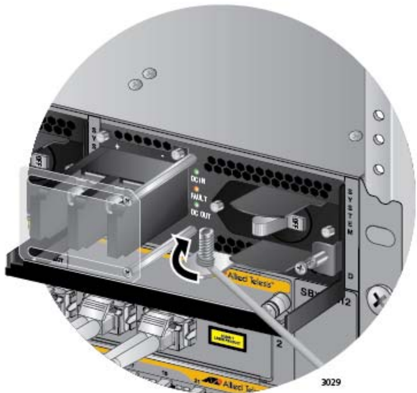
Figure 102. Attaching the Bare Grounding Wire to the Grounding Post
