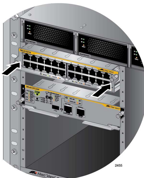
Figure 69. Seating an Ethernet Line Card on the Backplane Connector
