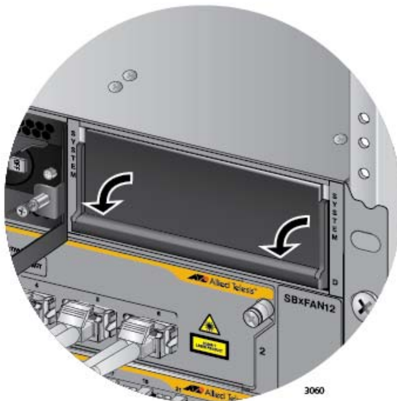
Figure 144. Lowering the Locking Handle on the Power Supply Slot Cover
