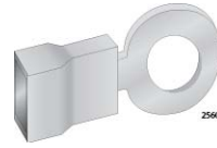
Figure 96. Grounding Wire Terminal
