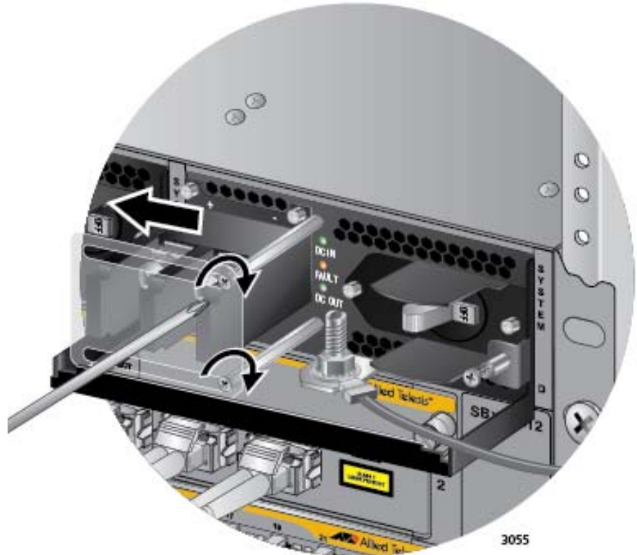
Figure 139. Closing the Plastic Cover
