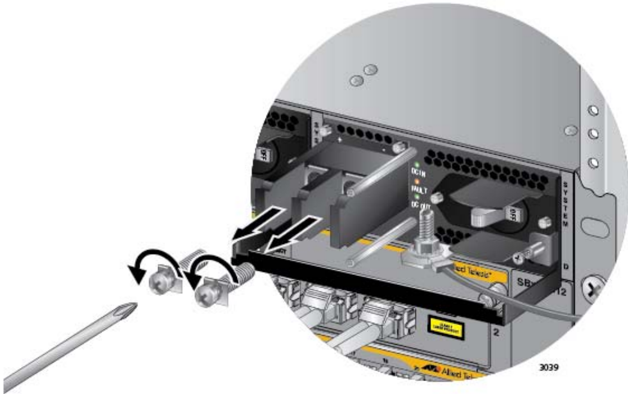
Figure 117. Removing the Terminal Screws
