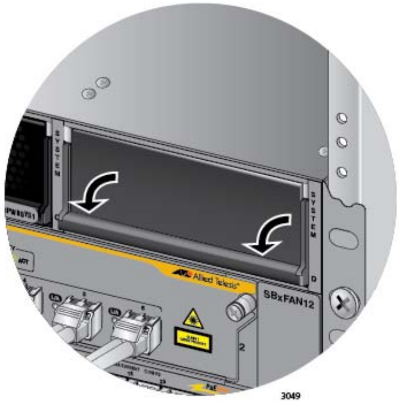
Figure 133. Lowering the Locking Handle on the Power Supply Slot Cover
