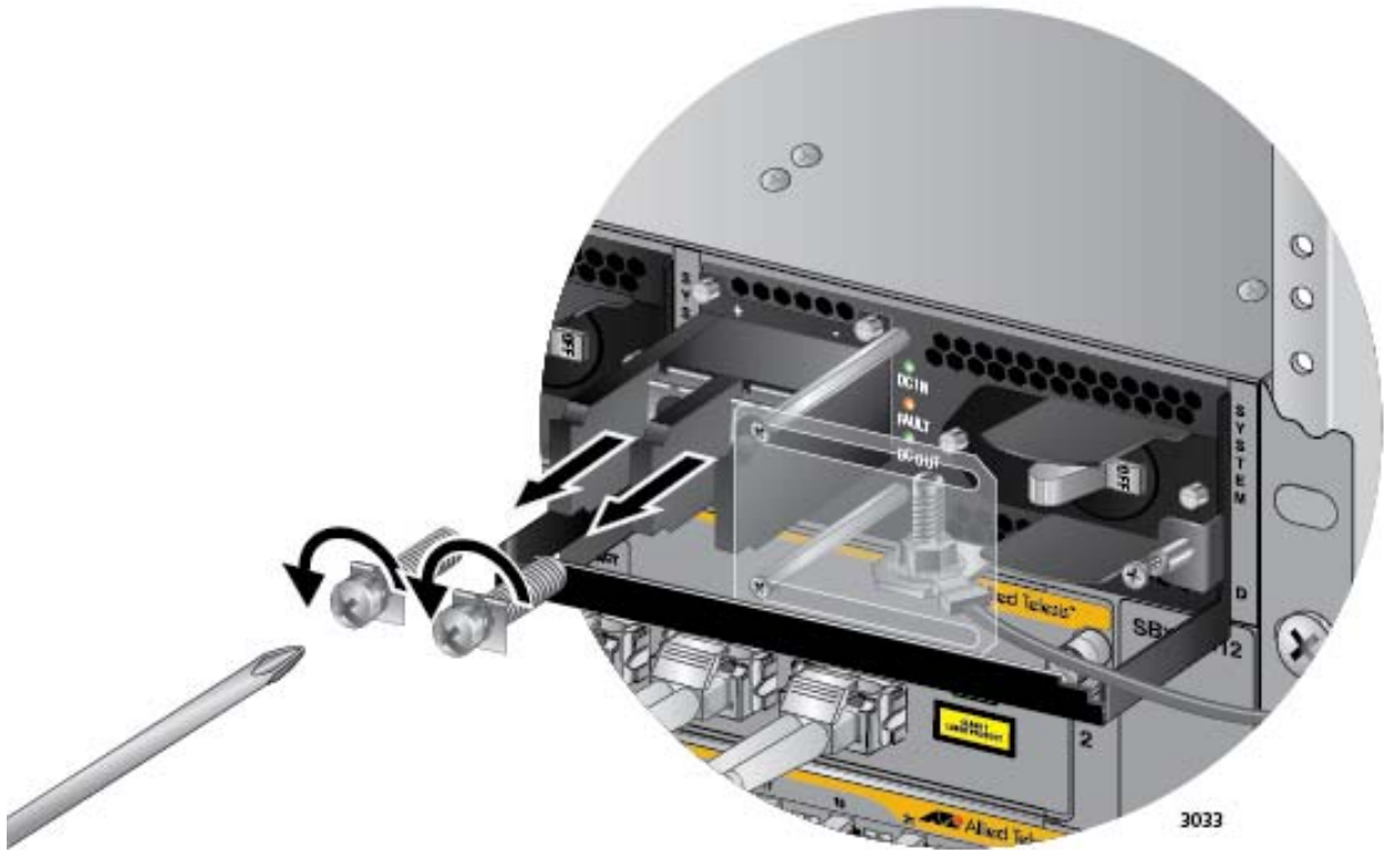
Figure 109. Removing the Terminal Screws
