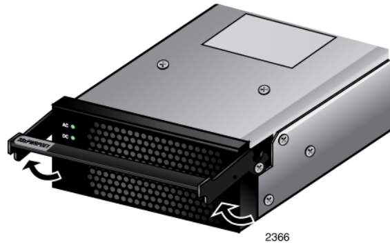
Figure 47. Unlocking the Handle on the AT-SBxPWRPOE1 Power Supply
