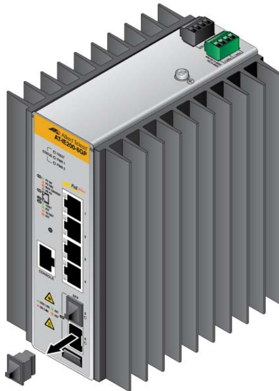
Figure 12: Removing the dust plug from an SFP slot.
