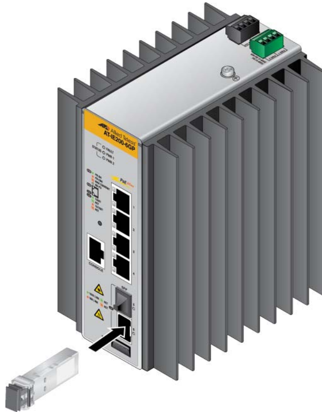
Figure 13: Installing an SFP transceiver.
