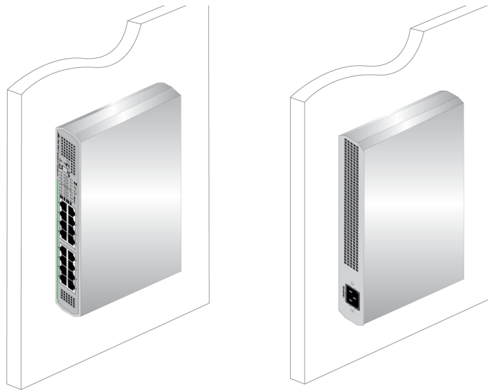
Figure 17. Correct Wall Installation for the AT-GS910/16 Switch
