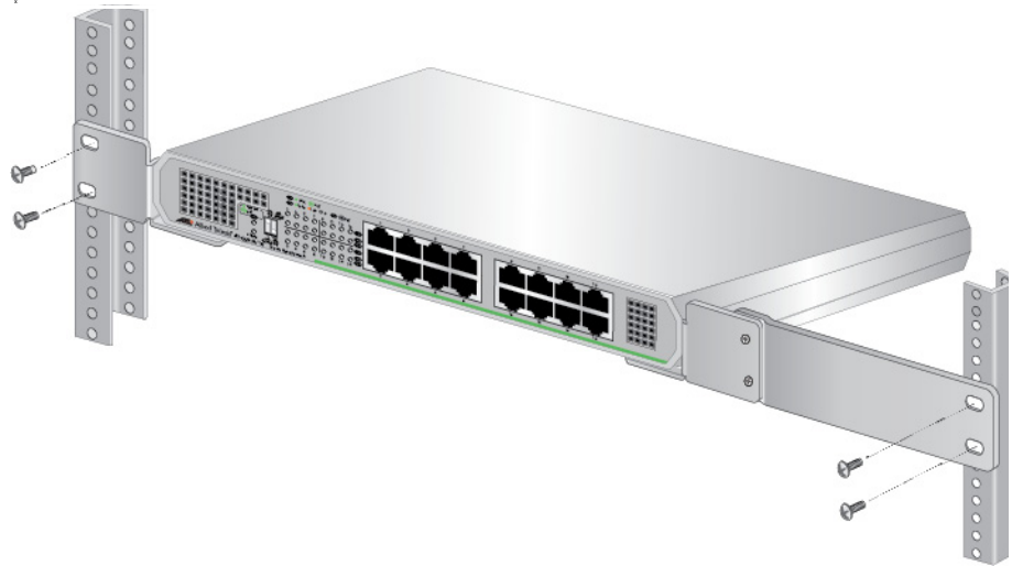
Figure 28. Attaching the Switch to an Equipment Rack
