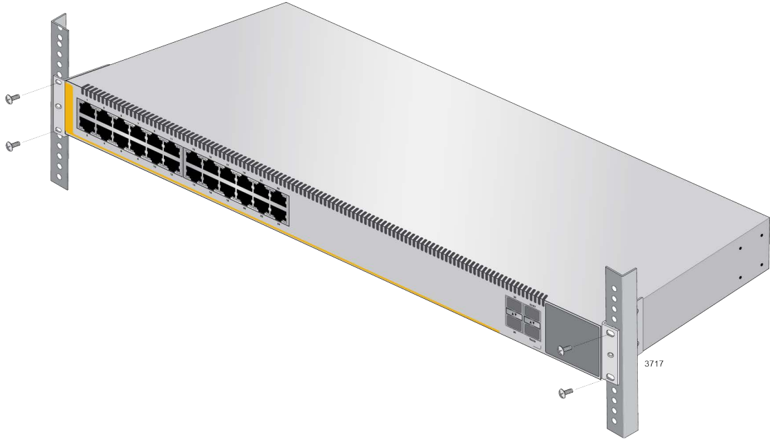
Figure 42. Installing the Switch in an Equipment Rack
