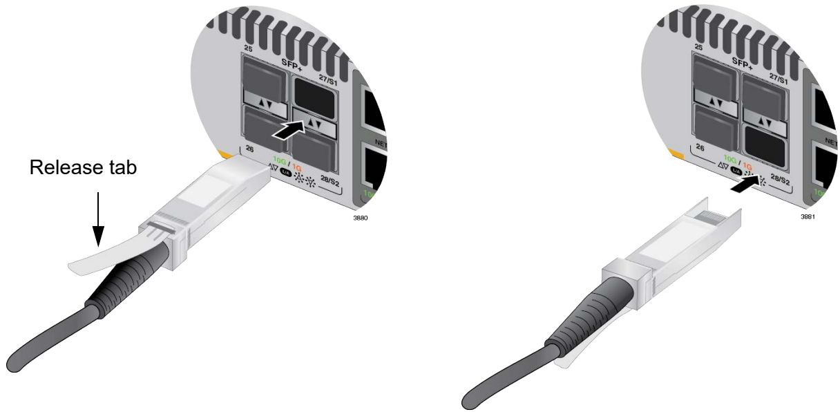
Figure 79. Installing AT-SP10TW Cables
