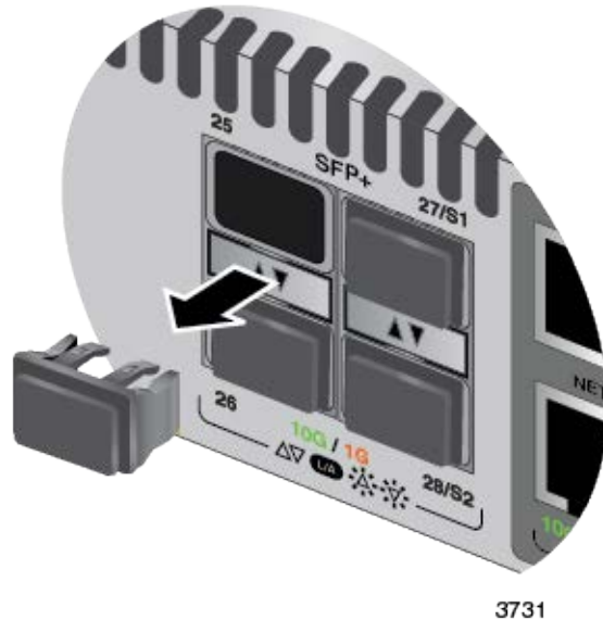
Figure 72. Removing the Dust Plug from an SFP Slot
