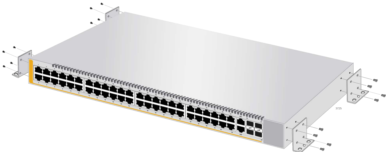
Figure 48. Installing the Brackets to the Switch for Wall Installation
