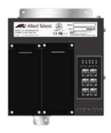
management. The modular design of the iMG 7x6 enables flexible configuration and provisioning by the service provider of the uplink and home networking slots.
