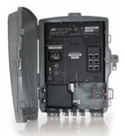
The iMG 7x6 outdoor fiber gateways are functional replacements for the popular iMG 6x6 products, incorporating a number of new features and enhancements. The AT-iMG 726MOD electronics feature two FXS voice ports supporting POTS or VoIP (SIP and MGCP), along with six 10/100 TX Ethernet ports. The AT-iMG 746MOD is identical, with four FXS ports. Both models use the same weatherproof outdoor enclosure designed to mount on the side of the home, with a separate splice tray and cable
