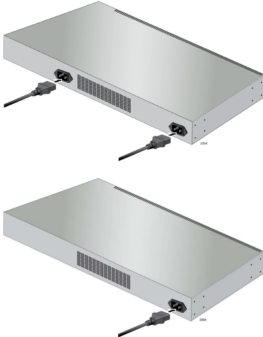
Figure 59. Plugging in the AC Power Cords
