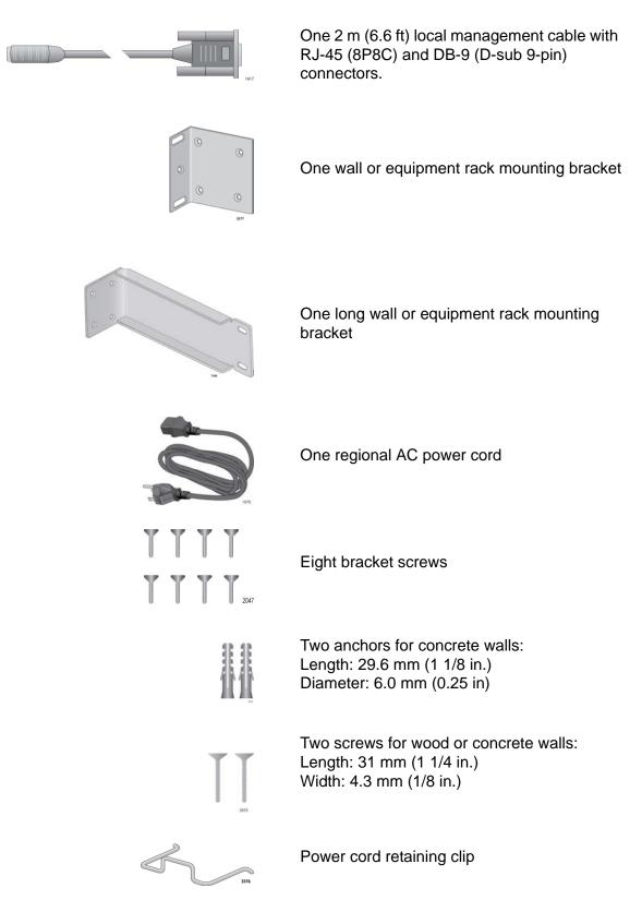
Figure 16. Components of the AT-x310-26FT Switch
