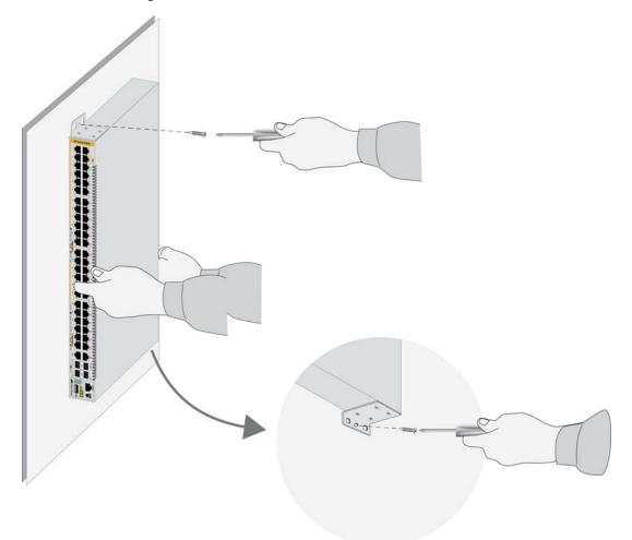
Figure 39. Installing the AT-x310-26FP, AT-x310-50FT, or AT-x310-50FP Switch on a Wall
