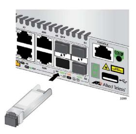
Figure 41. Installing an SFP Transceiver
