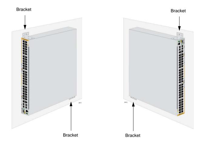
Figure 32. Bracket Positions on the Switch
