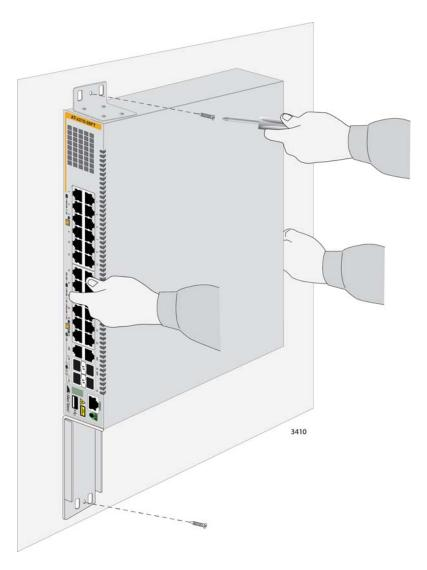
Figure 28. Installing the AT-x310-26FT Switch on a Wall
