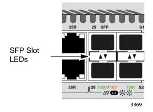
Figure 11. SFP Slot LEDs
