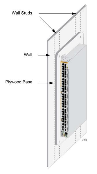
Figure 33. Switch on a Plywood Base
