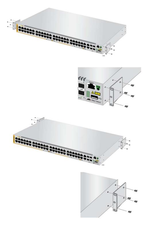
Figure 20. Attaching Brackets to the AT-x310-26FP, AT-x310-50FT, and AT-x310-50FP Switches
