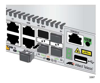
Figure 40. Removing the Dust Plug from an SFP Slot
