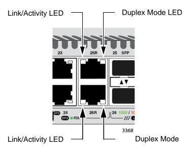
Figure 10. LEDs for the 10/100/1000Base-T Ports
