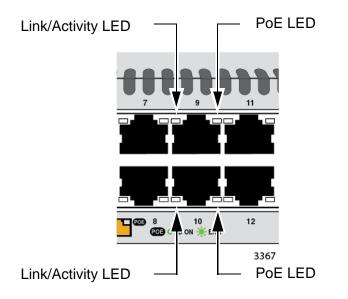
Figure 9. LEDs for the PoE 10/100Base-TX Ports on the AT-x310-26FP and AT-x310-50FP Switches
