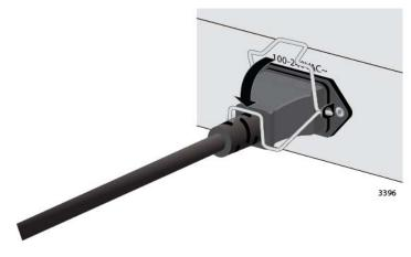
Figure 48. Lowering the Retaining Clip
