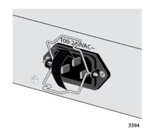
Figure 46. Raising the Retaining Clip
