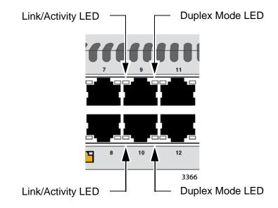
Figure 8. LEDs for the 10/100Mbps Ports on the AT-x310-26FT and AT- x310-50FT Switches
