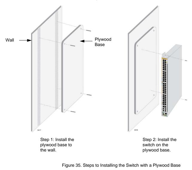
You should install the plywood base to the wall and then install the switch on the base. Refer to Figure 35.
