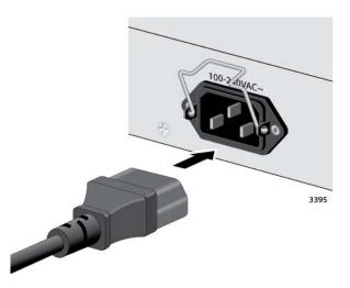
Figure 47. Plugging in the AC Power Cord
