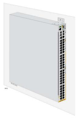
Figure 29. Positions of the AT-x310-26FP, AT-x310-50FT, and AT-x310-50FP Switches on a Wall
