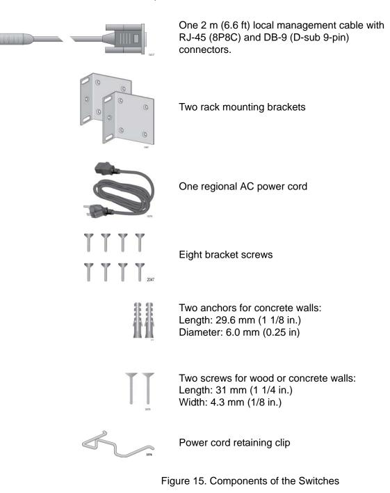
The AT-x310-26FT Switch comes with the components shown in Figure 16 on page 54.
