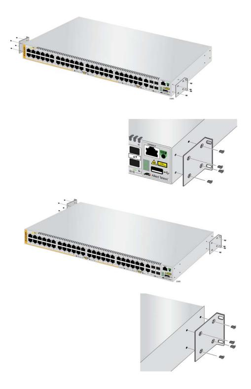
Figure 21. Attaching Brackets to the AT-x310-26FP, AT-x310-50FT, and AT-x310-50FP Switches (Continued)
