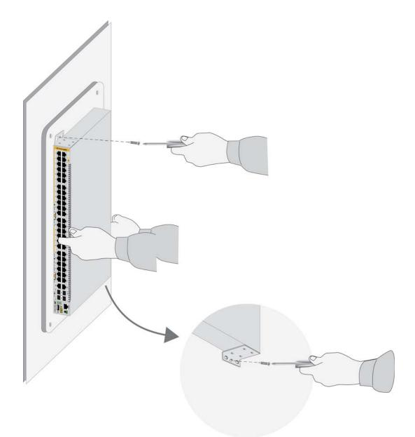
Figure 37. Securing the Switch to the Plywood Base
