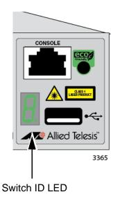
Figure 12. Switch ID LED
