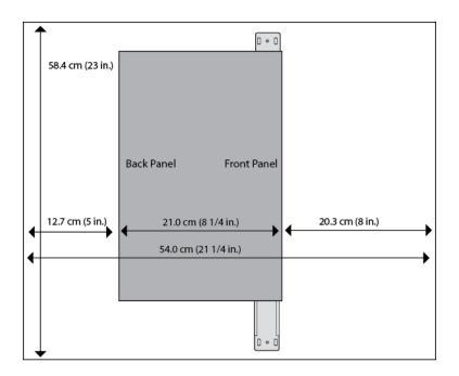
Figure 25. Minimum Wall Area Dimensions for the AT-x310-26FT Switch with the Front Panel on the Right
