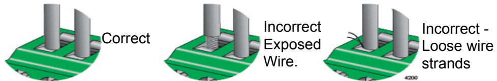
Figure 41. Verify Wire Installation
