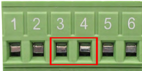
FIGURE 2-5 Fault Alarm Contacts
