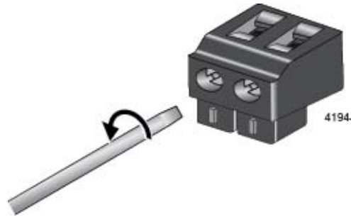
Figure 38. Loosening the Wire Retaining Screws on an Alarm Connector
