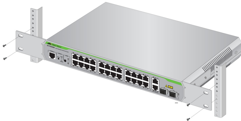
Figure 13. Mounting the Switch in an Equipment Rack
