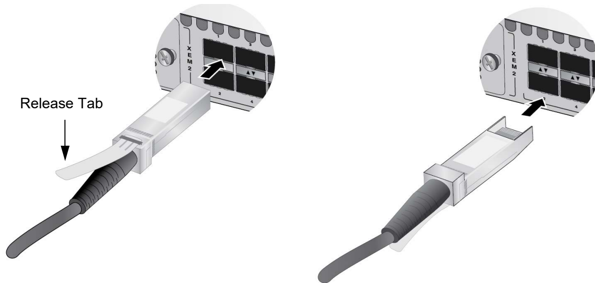
Figure 138. Installing SP10TW Direct Attach Cables
