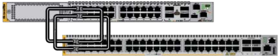
Stack of Two Switches
