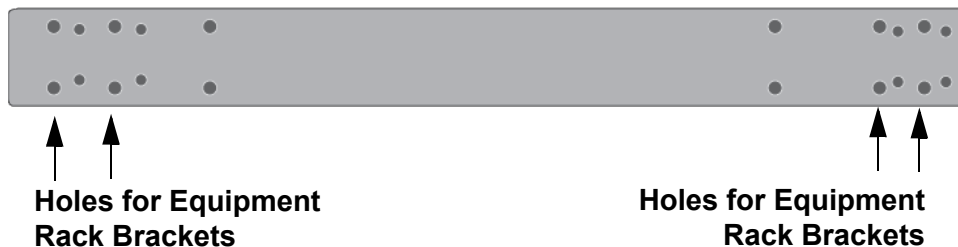
Figure 87. Holes for the Equipment Rack Brackets on the x950-52XSQ and x950-52XTQm Switches
