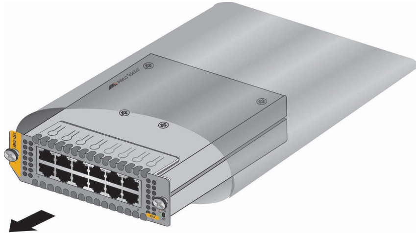
Figure 77. Removing the Ethernet Line Card from the Anti-static Bag
