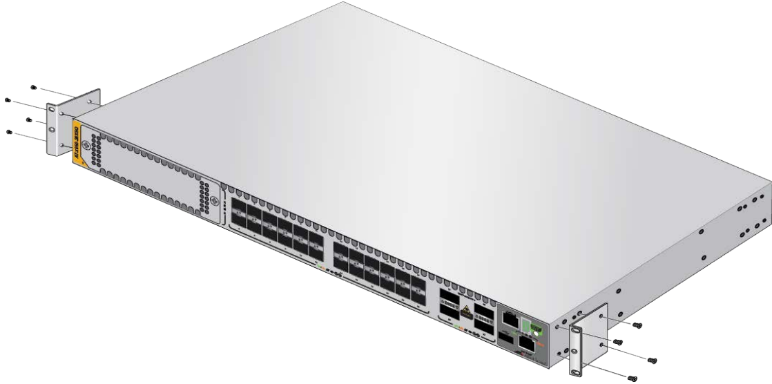
Figure 90. Attaching the Equipment Rack Brackets
