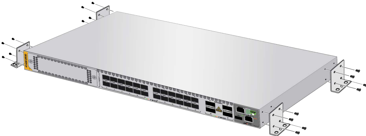
Figure 97. Installing the Brackets to the Switch for Wall Installation
