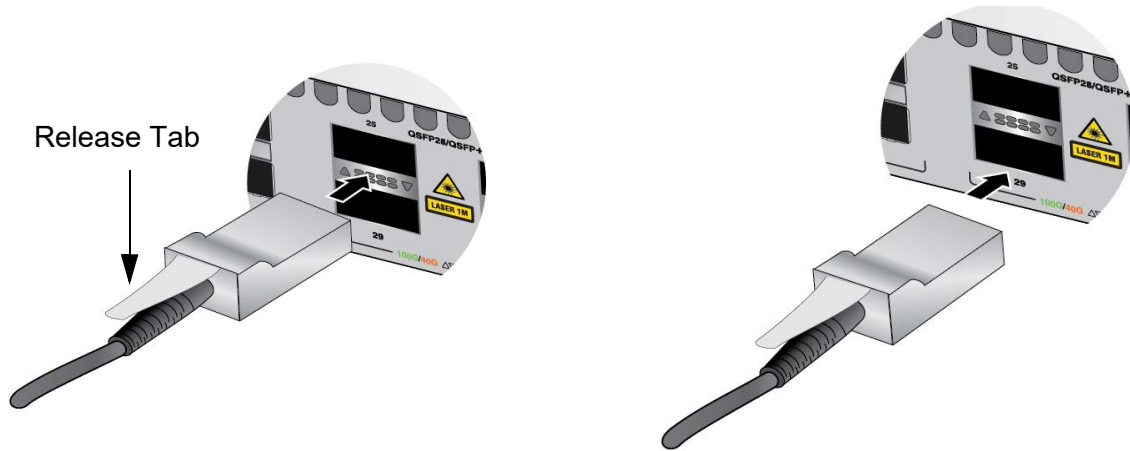
Figure 139. Attaching QSFP-CU Cables
