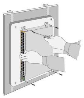
Four screws for the AT-x220-52GT or AT-x220-52GP Switch
