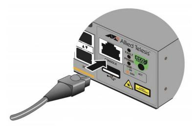
Figure 41. Connecting the Management Cable to the Console RS-232 Port
