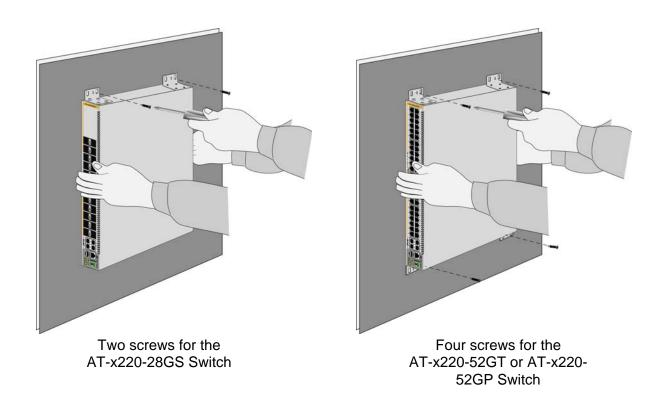
Figure 31. Installing the Switch on a Concrete Wall
