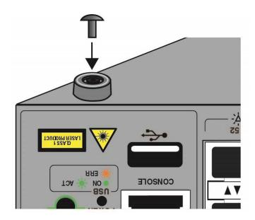
Figure 18. Inserting the Rivet into the Bumper Foot
