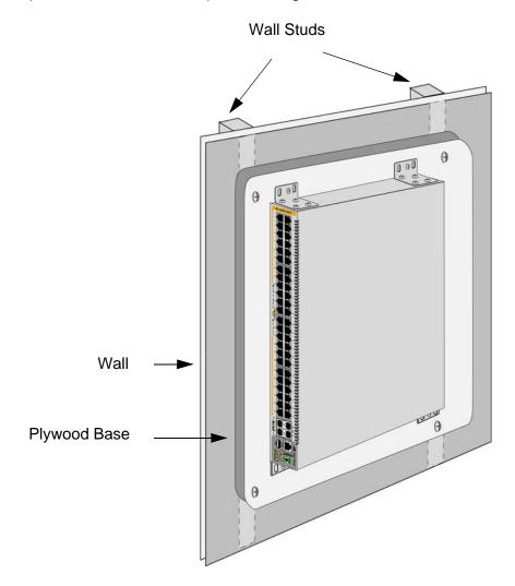
Figure 25. Switch on a Wall with a Plywood Base
