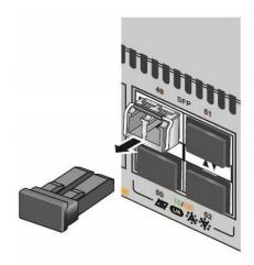
Figure 34. Removing the Dust Cover from an SFP Transceiver
