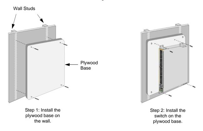
Figure 26. Steps to Installing the Switch with a Plywood Base
