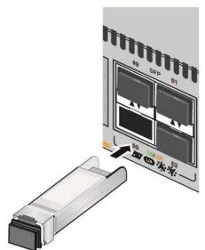
Figure 33. Installing an SFP Transceiver
