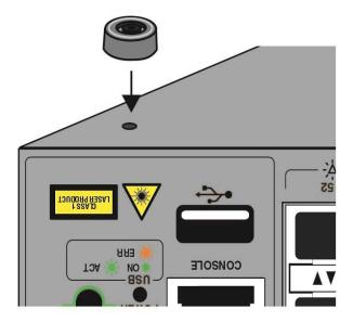
Figure 17. Place the Bumper Foot on a Base Corner Hole
