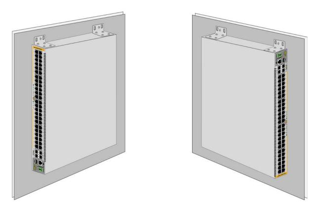
Figure 24. Positioning the Switch on the Wall
