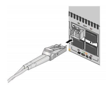
Figure 36. Connecting a Fiber Optic Cable to an SFP Transceiver
