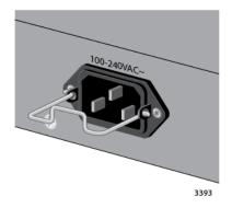
Figure 37. Installing the Power Cord Retaining Clip
