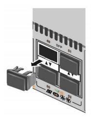
Figure 32. Removing the Dust Plug from an SFP Port
