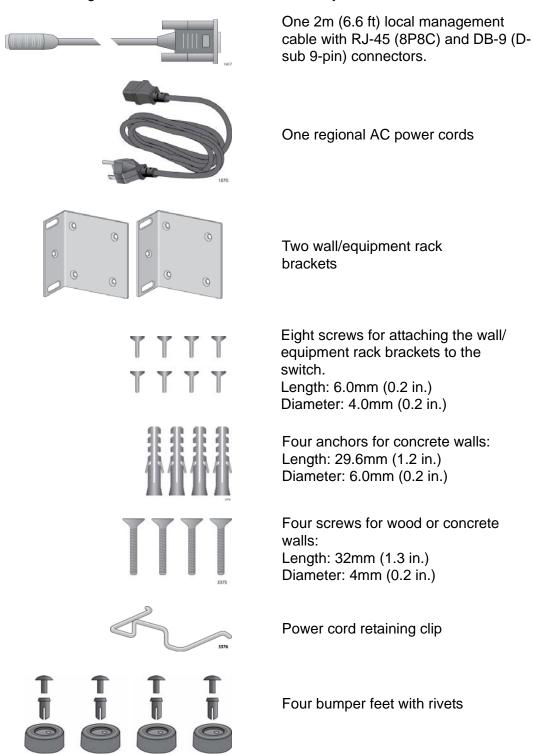
Figure 13. Accessory Kit for the AT-x220-28GS Switch
