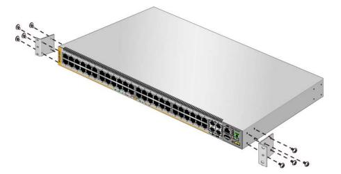
Figure 22. Example of Attaching the Brackets to the Switch
