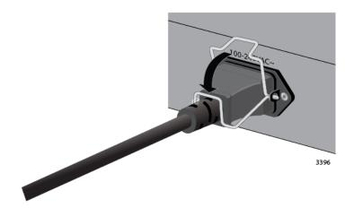
Figure 39. Lowering the Power Cord Retaining Clip
