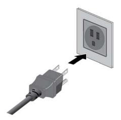
Figure 40. Connecting the Power Cord to an AC Power Source
