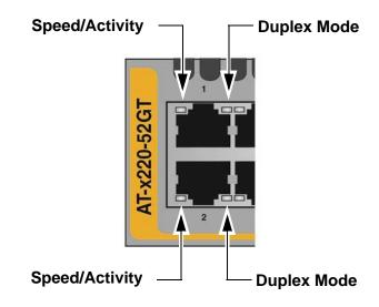
Figure 4. LEDs for the Twisted Pair Ports on the AT-x220-52GT Switch
