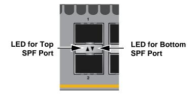
Figure 6. SFP Transceiver Ports LEDs
