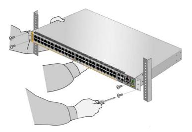
Figure 23. Installing the Switch in an Equipment Rack
