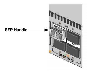
Figure 35. Positioning the SFP Handle in the Upright Position
