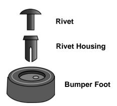
Figure 15. Parts of the Bumper Feet
