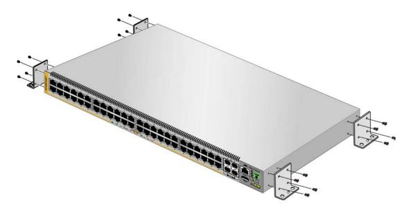
Figure 28. Bracket Positions for Installing the AT-x220-52GT or AT-x220-52GP Switch on a Wall
