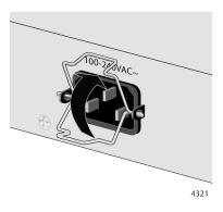
Figure 37. Raising the Retaining Clip
