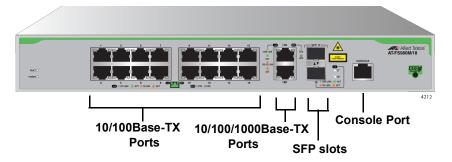
Figure 5. AT-FS980M/18 Switch Front Panel
