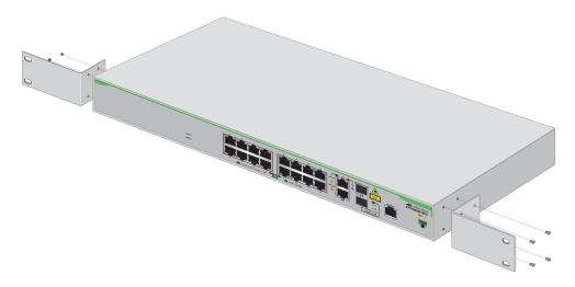
Figure 31. Attaching the Equipment Rack Brackets
