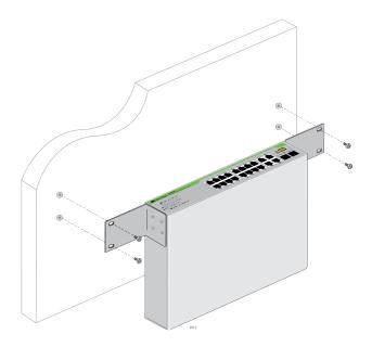
Figure 30. Driving the Screws through the Holes
