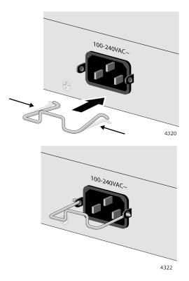
Figure 36. Installing the Retaining Clip
