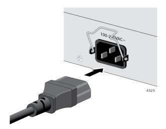
Figure 38. Plugging in the AC Power Cord
