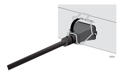
Figure 39. Lowering the Retaining Clip
