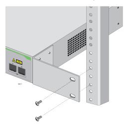
Figure 32. Mounting the Switch in an Equipment Rack
