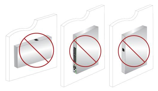
Figure 26. Incorrect Wall Installation
