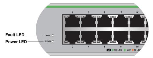
Figure 21. System LEDs
