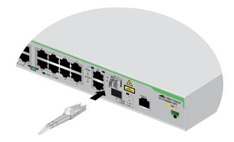
Figure 35. Connecting the Fiber Optic Cable to the SFP Module
