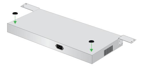
Figure 28. Attaching the Rubber Feet
