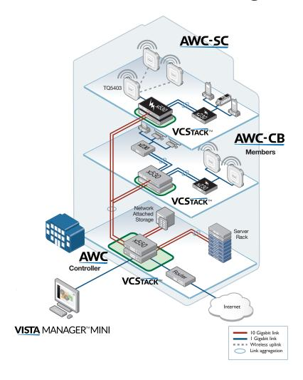
Allied Telesis Autonomous Wave Controller (AWC) offers solutions for two of the most common problems with Wireless LANs: initial setup complexity and on-going performance degradation. Initial WLAN set-up usually requires a site survey to achieve the best coverage; and performance of WLANs can often change over time as external sources of radio interference reduce coverage and bandwidth. These issues can be time-consuming to identify and resolve.
