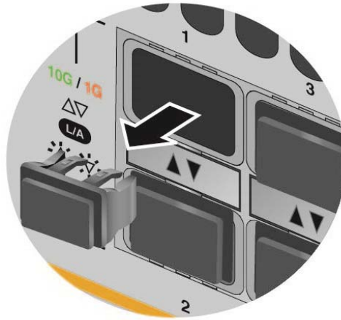
Figure 67. Removing the Dust Plug from an SFP Slot
