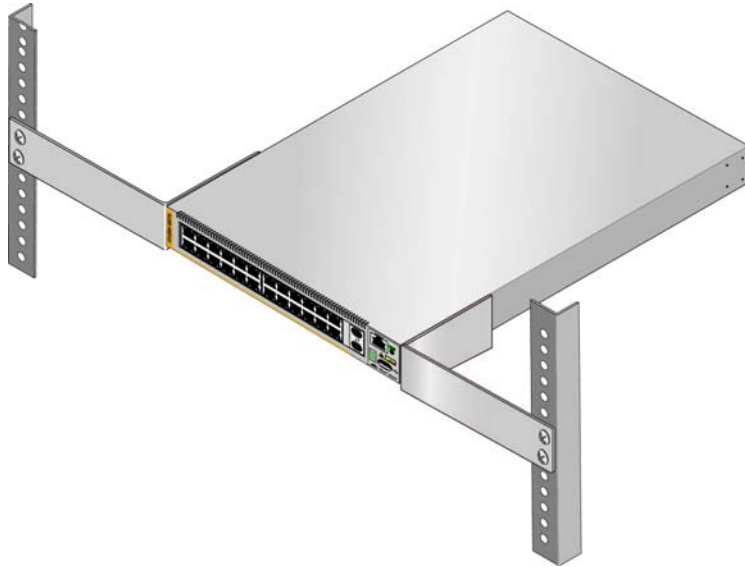
Figure 14. AT-RKMT-J14 Brackets and Switch
