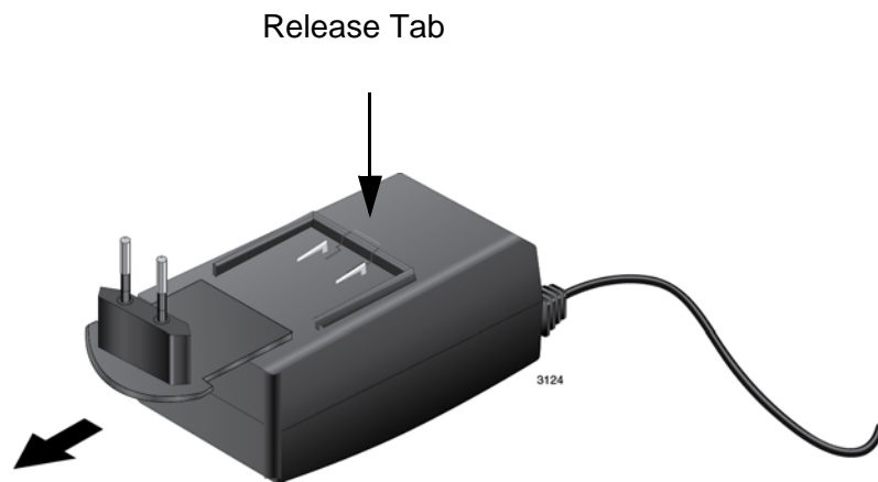
Figure 13. Removing an AC Plug from the AT-TQ0091 AC/DC Power Adapter
