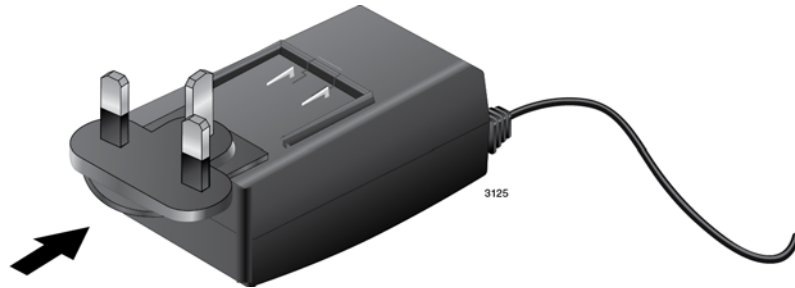
Figure 14. Installing an AC Plug on the AT-TQ0091 AC/DC Power Adapter
