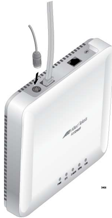
Figure 12. Connecting the Power Cable from the AT-TQ0091 AC/DC Adapter
