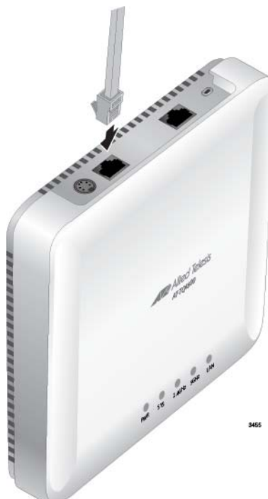
Figure 11. Connecting the Network Cable
