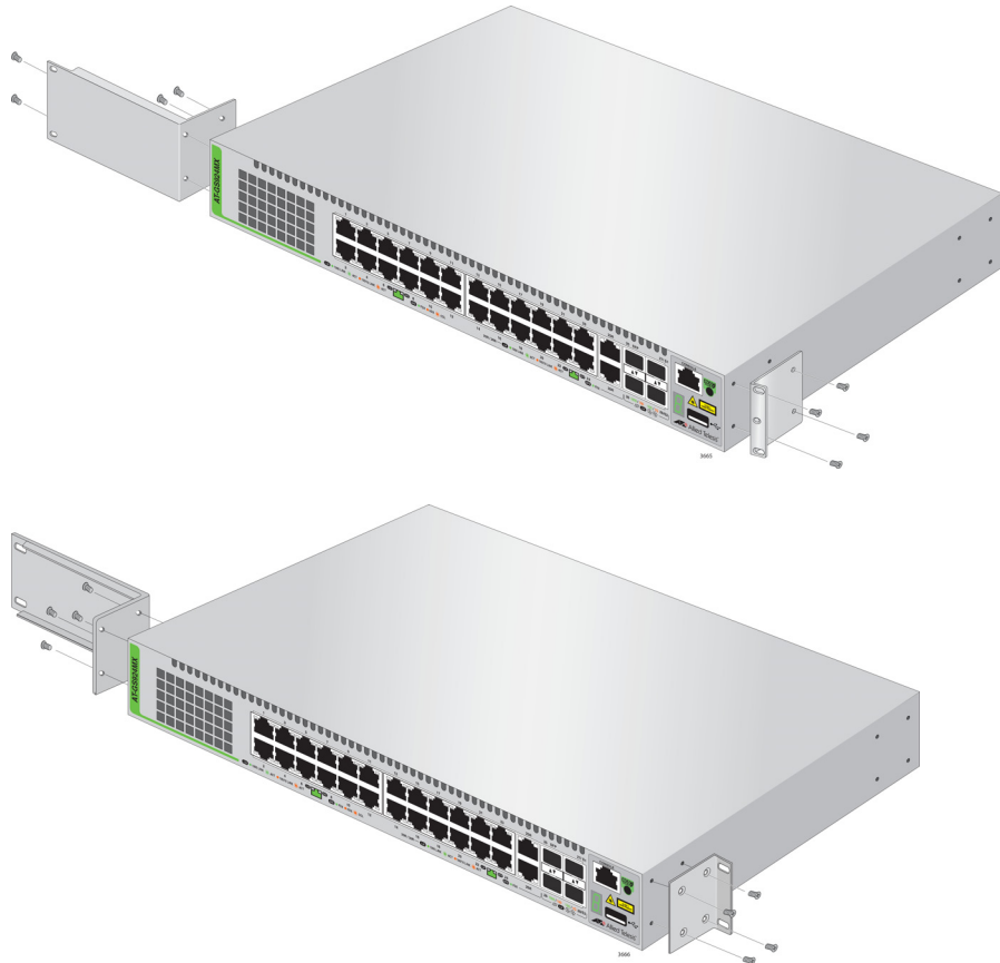
Figure 19. Installing Brackets on the AT-GS924MX Switch
