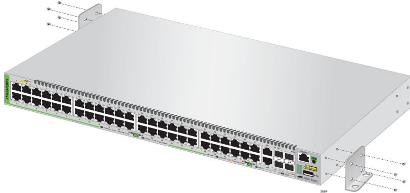
Position of the brackets if the switch is to be installed on the wall with the front panel on the right.
