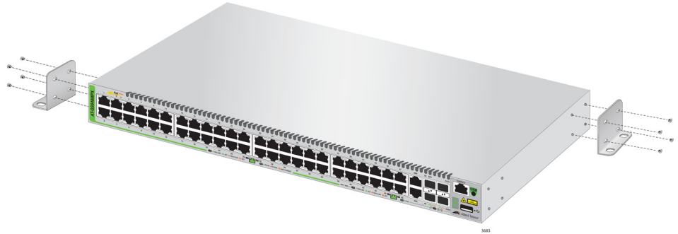
Positions of the brackets if the switch is to be installed on the wall with the front panel on the left.
