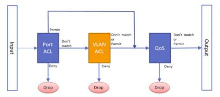
On these switches, once an ACL denies a packet, the switch stops checking against futher ACLs and drops the packet. If a port ACL permits the packet, the switch does not check VLAN ACLs. If either a port ACL or VLAN ACL permits the packet, the switch checks the packet against QoS ACLs.
