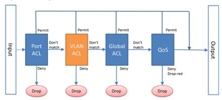
Once a packet matches an ACL (either a permit or deny match), the SBx908 or SBx8100 switch stops checking it against further ACLs.
