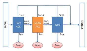
Once a packet matches an ACL (either a permit or deny match), the IE200 Series switch stops checking it against further ACLs.
