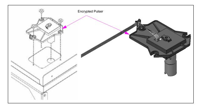
This pulser is not intended for use with Encore 500/S/700 S/S E-CIM units for Ultra-Hi Flow (UHF), DEF, or installed with Ecometer.
