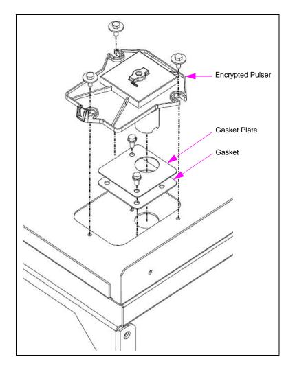
The M12514K002 and M12514K003 Assemblies are the same as M12514K001, except for the removal of the old gasket, and reassembly of a new pulser drive gasket and plate.
