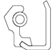
SC / A Profile Oil Seal 7 PSI - Single Lip
