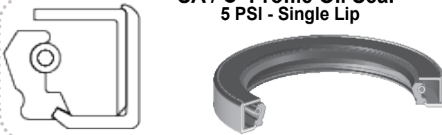
SB Profile Oil Seal 5 PSI - Single Lip
