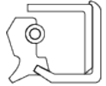
TB Profile Oil Seal 5 PSI - Double Lip
