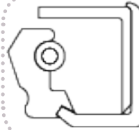
SB Profile Oil Seal 5 PSI - Single Lip
