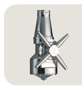
liquid in the tank. The nozzles rotate around both the horizontal and vertical axes in a 360° movement. This three-dimensional jet rotation enables the jets to reach the entire tank volume, providing fast, efficient mixing of the injected liquid, gas or powder without requiring batch rotation.
