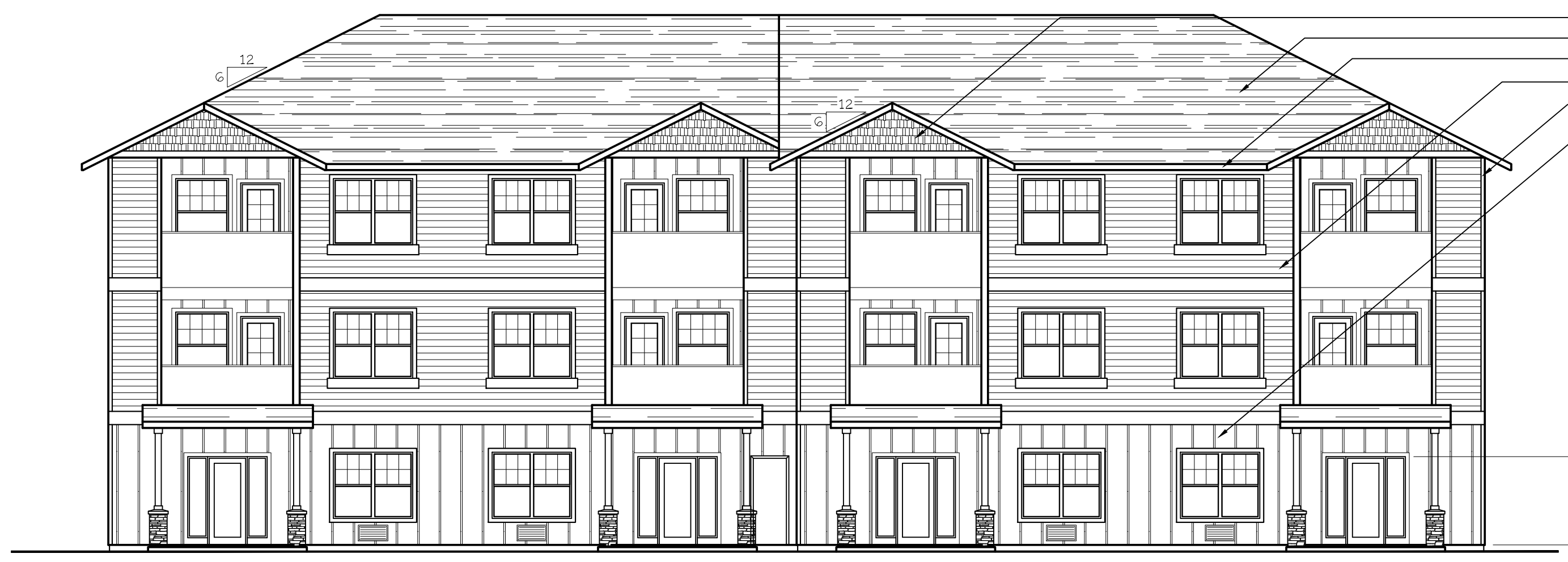
WEST ELEVATION (TYPE A UNITS) SCALE: 1/8" = 1'-0" BLD. 6
