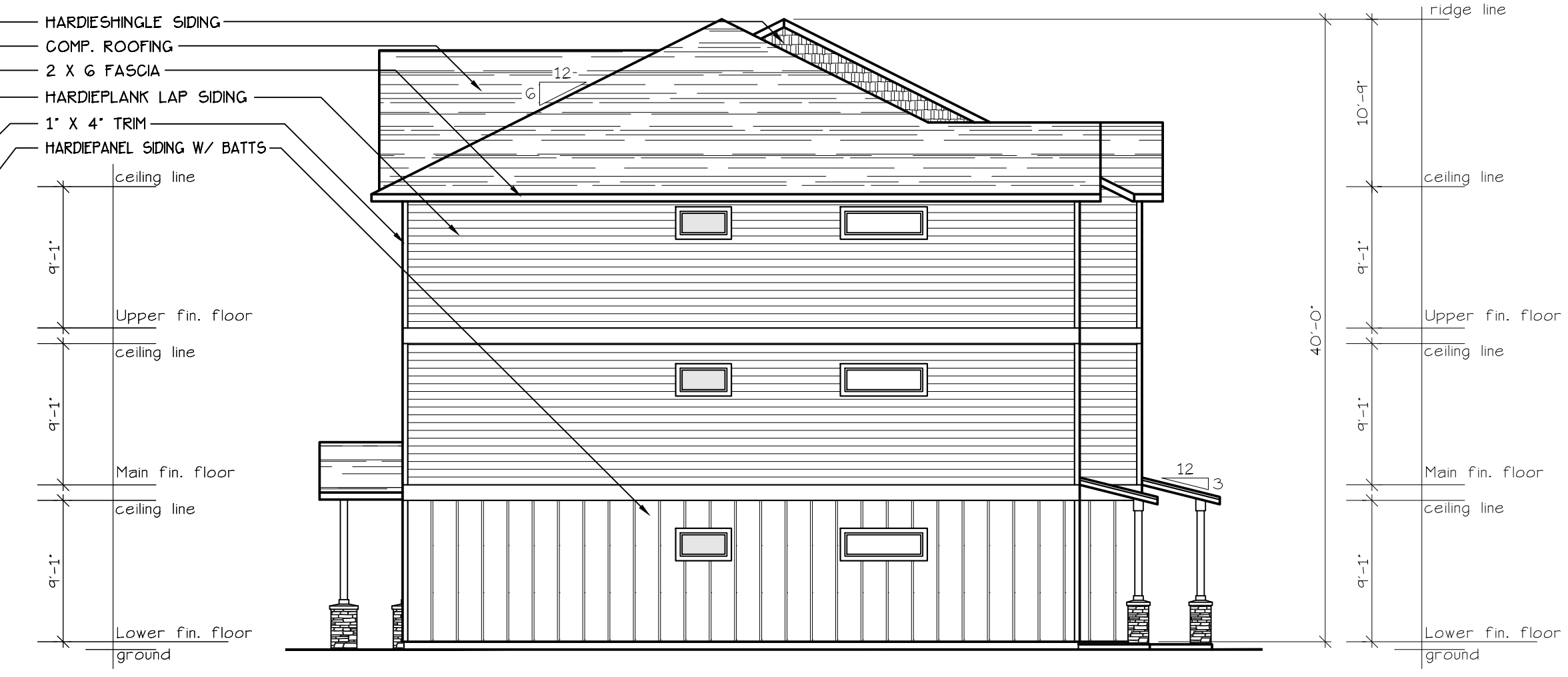
NORTH ELEVATION (TYPE A UNITS) SCALE: 1/8" = 1'-0" BLD. 6
