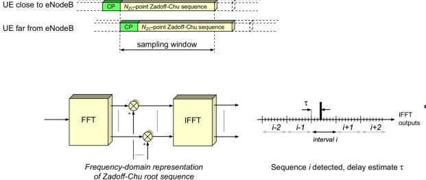
> Time domain output shows which of the shifts of the root Zadoff-Chu sequence has been transmitted and its delay
