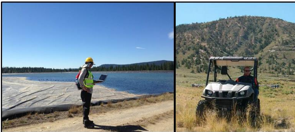
Figure 1 Mobile GPS Integrated Gamma Survey System – Backpack (left) and ATV (right)
