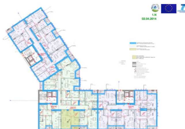
Figure 7: Airtightness sectors C-1 (apartments C-1-1, C-1-2, C-1-3, C-1-4), B-1, A-1 covering three staircases of the 1 st floor of the residential part.
