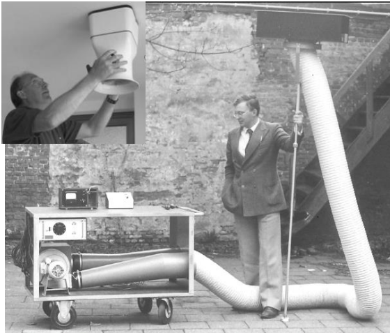
Figure 3: two zero pressure measuring systems, one from 1978 and one as it is being built today (top left)
