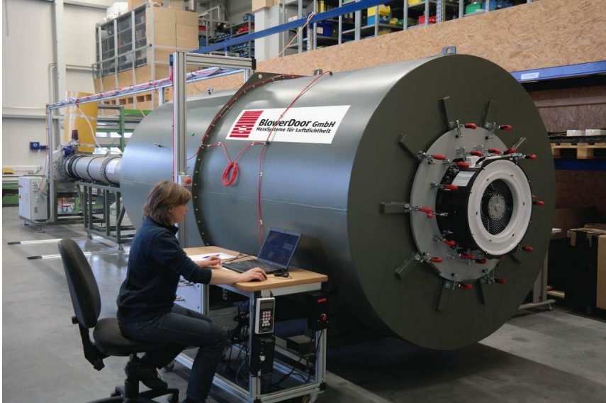
Figure 11: Calibration station for measuring flow rates with a BlowerDoor bellows gauge.
