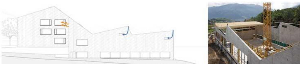
Figure 7. For winter natural ventilation strategy, air enters from the top lateral openings and goes out from the top front opening in order to avoid cold draughts. Cold air entering at 8 m height, is mixed with hot air until it falls to the floor. Users have not reported any cold draughts in the first year use of the gym.
