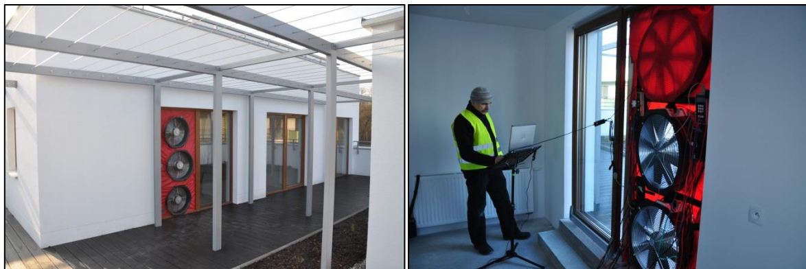
Figure 9: Minneapolis Blower Door set used for the tests
