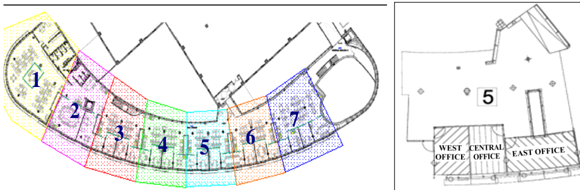
Figure 4: From left to right: Monitoring project design into seven areas, and detail of the office distribution on central areas.
