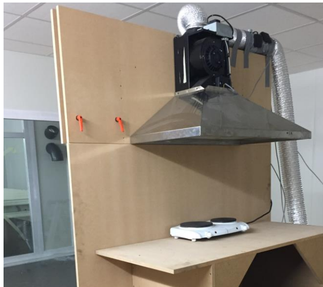
Figure 1: The experimental setup with adjustable range height, electric range and air curtain assisted range hood in wall mounted non-enclosed mode.
