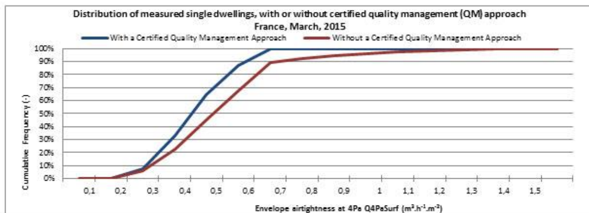
Figure 5: distribution of measured airtightness of houses with and without implementations of a certified QM approach
