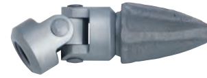
Drill Head with Universal Joint Range: 1-1/2 in. (38.1 mm) - 2-1/8 in. (53.9 mm) Deposit: light-hard to medium
