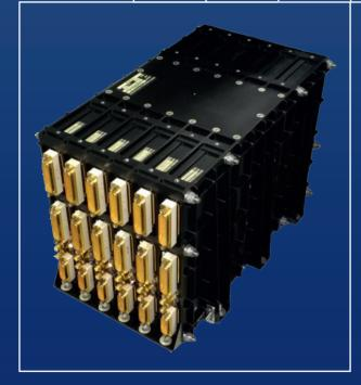
CORECI 2 is a high performance integrated COmpression, REcording and Clphering equipment for high-resolution Earth observation satellites.
