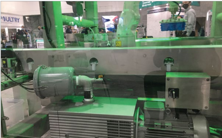
The OSSID E40 REEPACK Line featuring a built-in chiller, vacuum pump and compressed air powered vacuum venturis for the suction cups.
