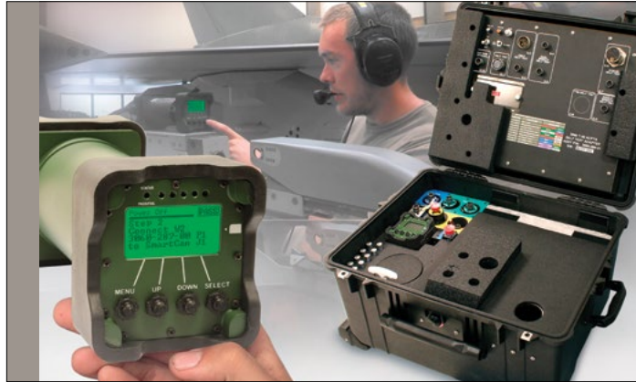
A Marvin Test Solutions MTS-3060A SmartCan Universal Armament Test Set with adapter and cable kit.
