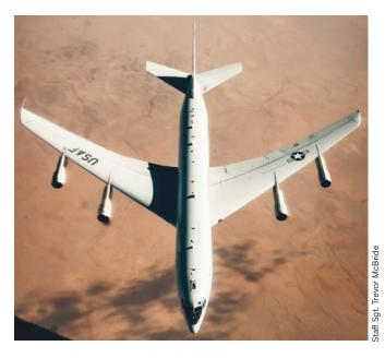
Link (SDL) for LOS networking to Common Ground Stations and FY21 launches UHF/VHF SATCOM modernization. USAF aims to re-engine the fleet with refurbished JT8D-219 turbofans as a cost-effective interim solution to improve performance and reliability.
