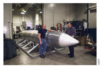
nine weeks to be available for the 2003 Iraq campaign. The weapon was designated Massive Ordnance Air Blast (MOAB) but is unofficially known as "Mother of All Bombs." The weapon is designed for deployment from the ramp of an MC-130 without a parachute. A total of 18,700 lb of the weapon's 21,000-lb weight is attributed to BLU-120/B warhead. It was used operationally for the first time in April 2017 against an ISIS-occupied cave complex in Afghanistan.
