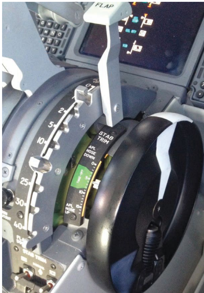
▲ A Boeing 737 MAX trim wheel. The autopilot stab trim cutout switches are at lower left.
