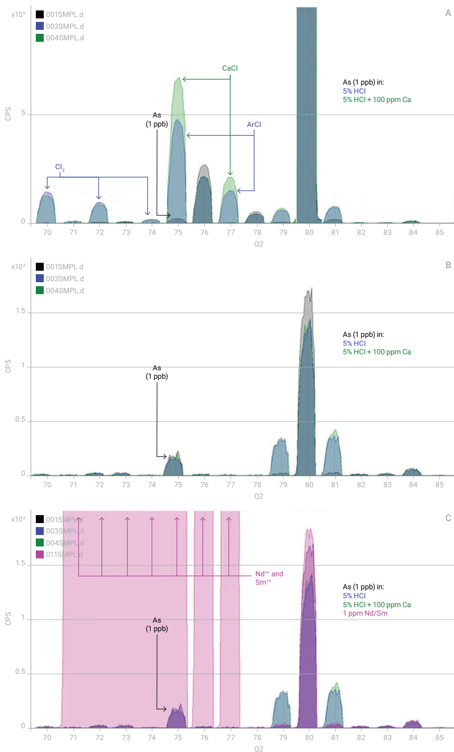
Figure 1. a) \text{As}^+ ( m/z 75) in no gas mode, showing polyatomic interferences from \text{ArCl}^+ and \text{CaCl}^+ ; b) \text{ArCl}^+ and \text{CaCl}^+ polyatomics are removed in He collision mode; c) He collision mode fails to remove \text{Nd}^{++} and \text{Sm}^{++} interferences at m/z 75.
