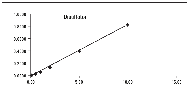
Figure 5. Correlation coefficients for the EPA Method 525.2 pesticide components over the 0.1 to 10 µg/mL range of this study and an example linear regression plot for disulfoton.
