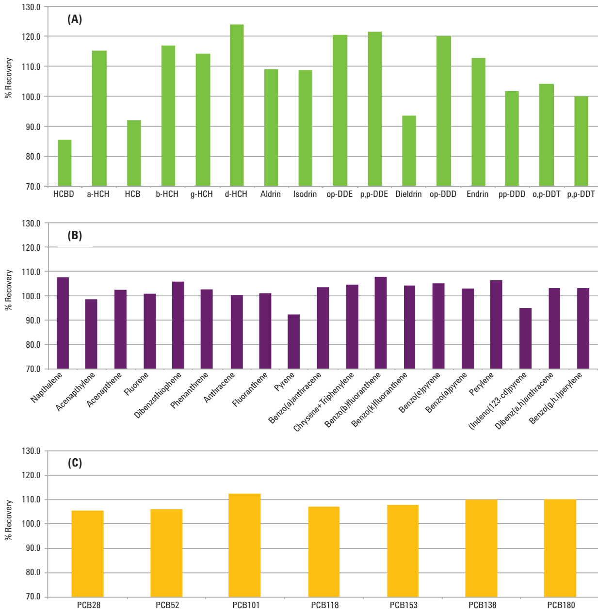
Figure 8. Graphical representation of analyte percent recovery values for (a) OCPs, (b) PAHs and (c) PCB congeners in spiked mussel tissue.
