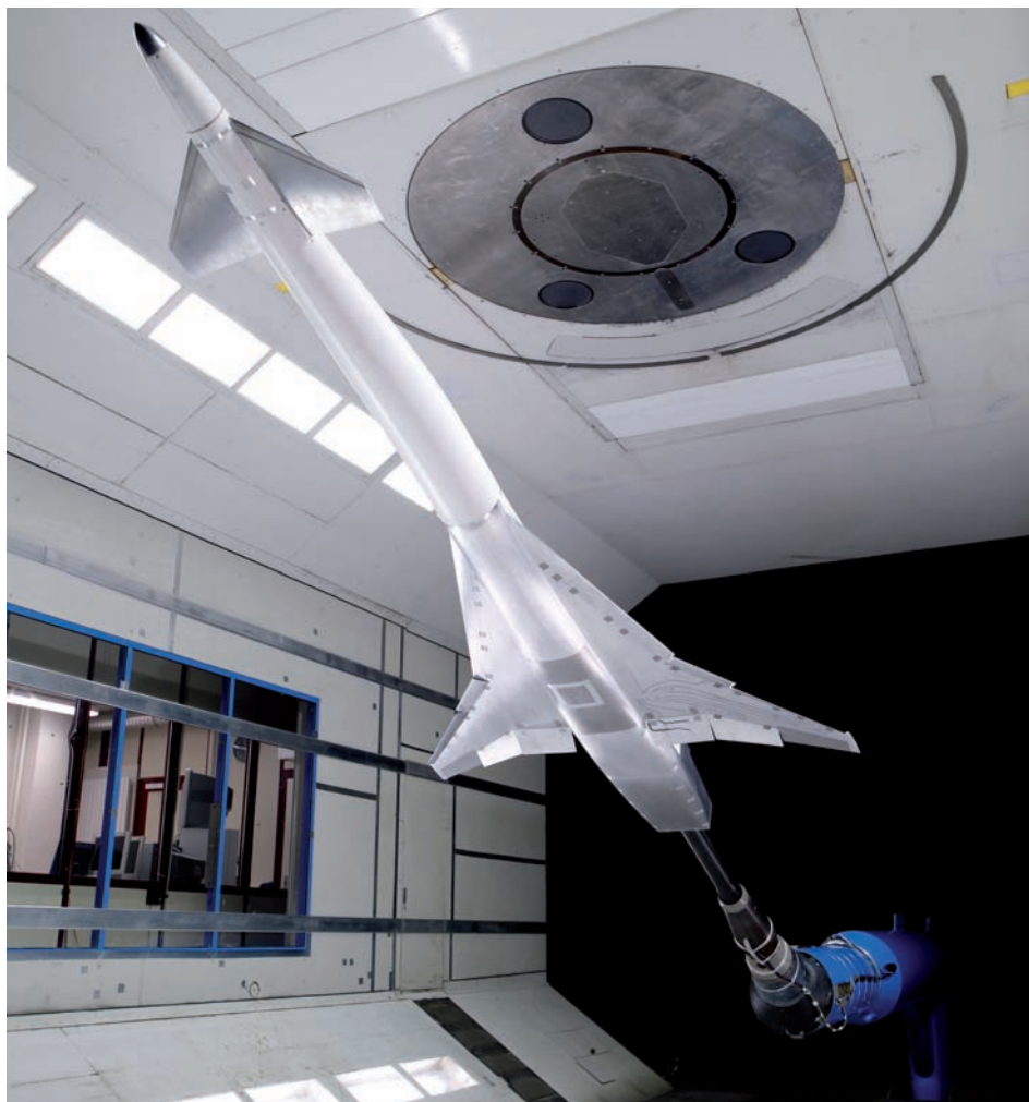
Above: The HISAC low-speed wind tunnel test at 68m/s
