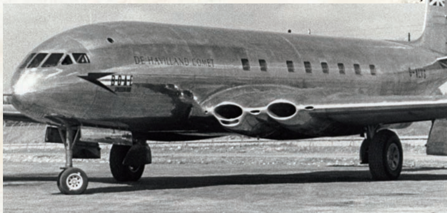
The Comet's thin metal skin was composed of advanced new alloys
