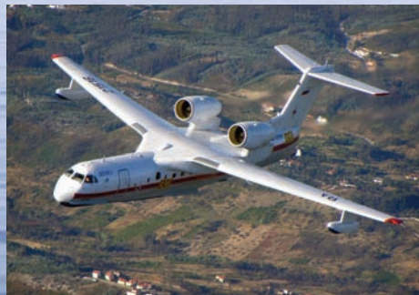
The multirole Be-200 can be configured as an amphibious water drop firefighting aircraft, a freighter, or as a passenger aircraft
