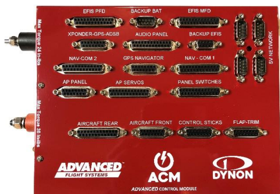
ACM module with Electronic Circuit Breakers
