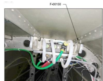
FIGURE 4: F-00150 DUAL ADAHRS INSTALL
