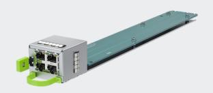
Advanced Energy's Artesyn PMI is an extension module, which brings MODBUS of the PSU/BBUs directly out for upstream communication. PMI sits on Open Rack V3 Power and Battery Shelves. On one end, it has communication with the PSU or BBUs – through sliver straddle connector. On the other end, interacts with centralized system through the use of RJ45 connectors.
