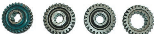
6 10 23 15 Four different female spline transfer case drive gears
