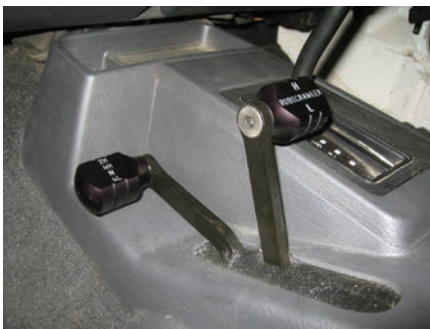
Jeep JK console (right) with the RubiCrawler twin stick shifter installed.
