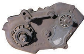
NP205 T/C figure-8 bolt pattern
