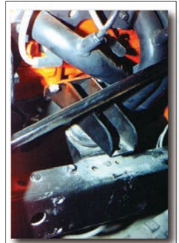
Photo illustrates motor mount installed with Saginaw steering conversion
