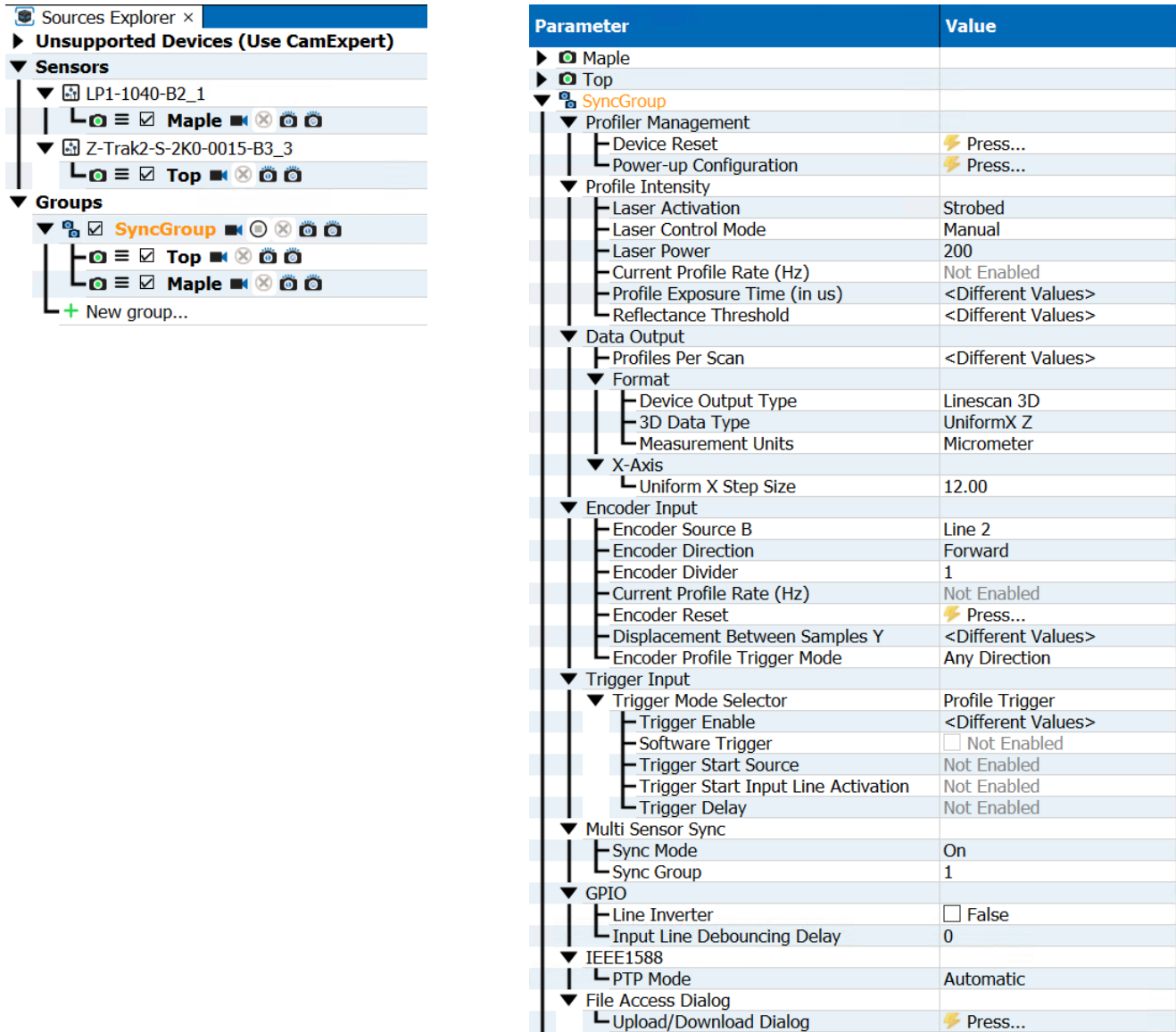
Figure 20. (Left) Sources Explorer with the SyncGroup. (Right) The Features Browser with all parameters that may be set for the group.
