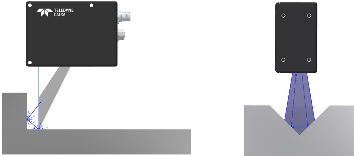
Figure 16. Reflective surfaces or objects with oddly angled surfaces may scatter the laser light back into the 2D sensor window, creating blurred profiles.
