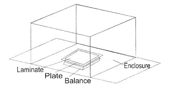
Figure 17.1. Typical Balance Enclosure
