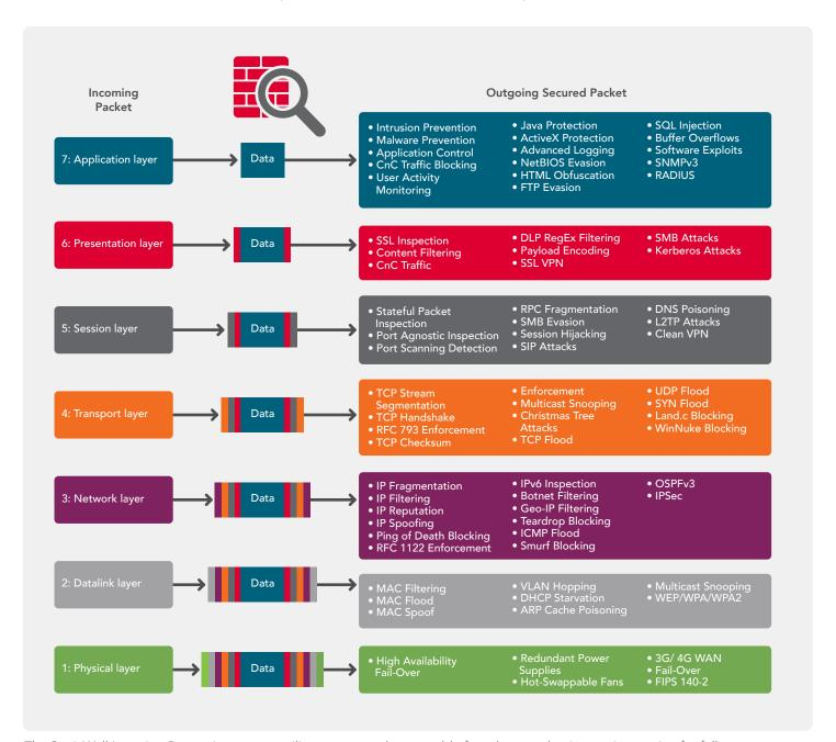
The SonicWall Intrusion Prevention system utilizes a patented reassembly-free deep packet inspection engine for full stack protection.
