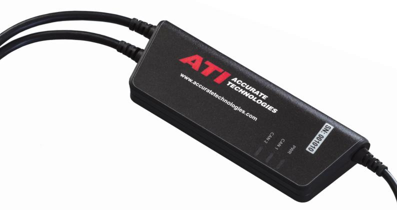
The ATI USBcan Pro 2xHS v2 is a USB to dual-channel CAN or CAN FD interface with advanced scripting capabilities. Featuring galvanic isolation, a standard USB connector and two high-speed ISO 11898-2 CAN channels, it is a high-performance yet compact, plug & play dual-channel interface, designed to connect a CAN bus network to a PC or mobile computer.
