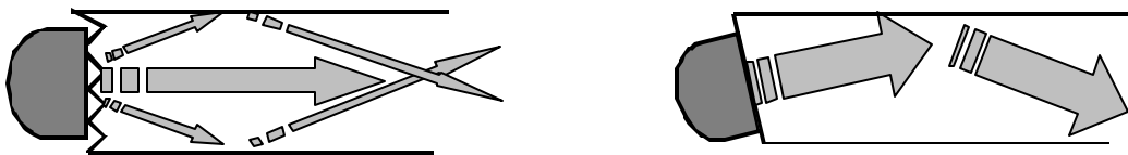
Figure 2 Rough and angled transducer contact
