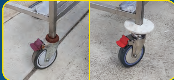
This bakery trolley has been upgraded with new grade 304 stainless steel castors
