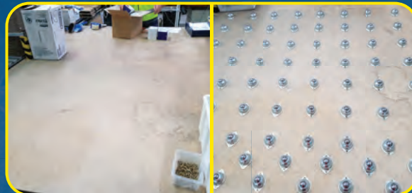
Stock transfer table refurbished with new rollers
