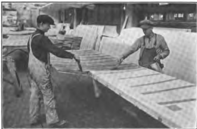
"DOPING" THE WINGS, THE TREATMENT FOR WATERPROOFING THE WING FABRIC AND MAKING IT NON-INFLAMMABLE
