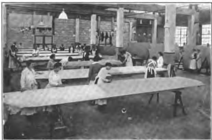
COVERING THE WINGS WITH FABRIC, DAYTON-WRIGHT AIRPLANE COMPANY, PLANT 1
