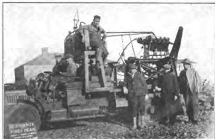
THE LIBERTY MOTOR AT THE SUMMIT OF PIKE'S PEAK FOR ITS FIRST ALTITUDE TEST, AUGUST, 1917
