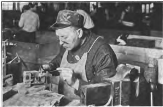
EXPERT WELDING ON CAPRONI FITTINGS, STANDARD AERO CORPORATION
