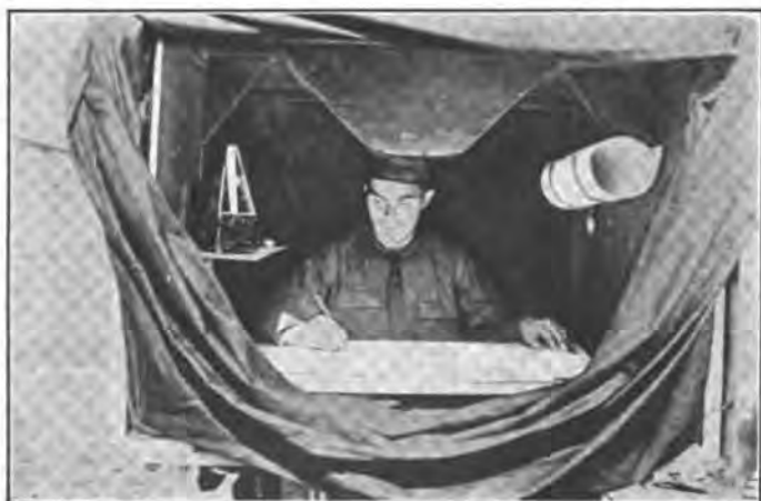
OBSERVER IN THE "CAMERA OBSCURA" USED ON BOMBING PLANES, IN WHICH, BY AN ARRANGEMENT OF LENSES AND MIRRORS, A PANORAMA OF EXTERNAL OBJECTS IS PROJECTED UPON A SHEET OF WHITE PAPER
