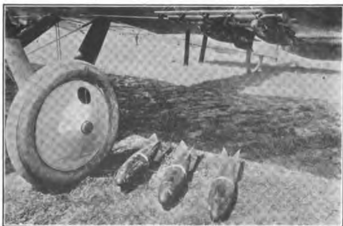
THE BOMBS AND THEIR RELEASING DEVICE
