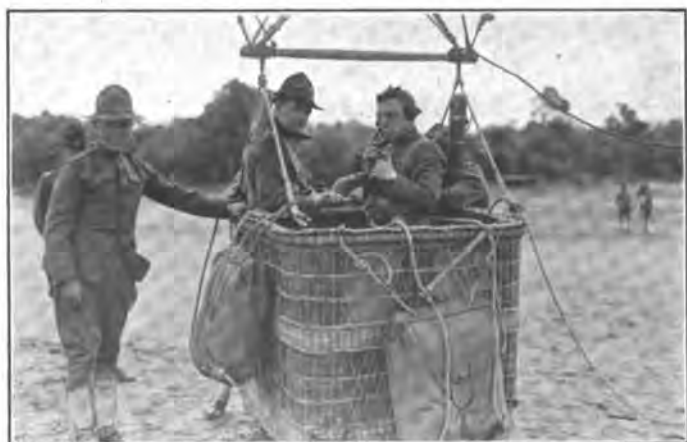
PILOT AND ARTILLERY OBSERVER IN BALLOON BASKET WITH TELEPHONE EQUIPMENT AND PARACHUTES IN STOPS; EACH PARACHUTE IS ATTACHED TO THE MAN WHO MAY HAVE TO USE IT
