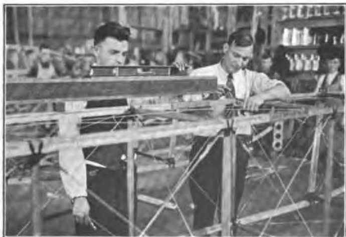
TRUEING UP THE FUSELAGE
