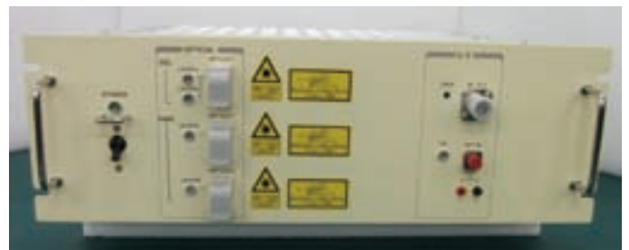
SHF Band Transmitting Unit (MTU-50N)
