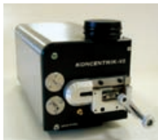
Patchcord concentricity + index measurement
